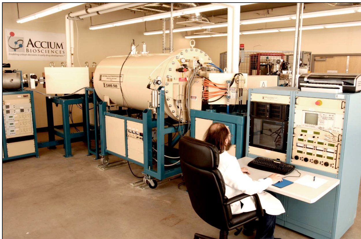
Dr. Ugo Zoppi operates Accium's 500,000-volt Accelerator Mass Spectrometer
