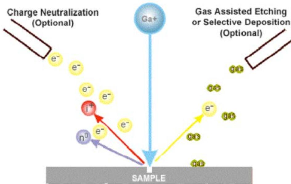
Figure 1: Diagram of the FIB process.
