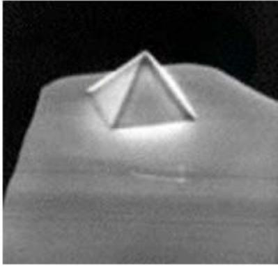
Figure 5: The pyramid structure of an AFM tip made using anisotropic wet etching of single crystal silicon. The tip of the pyramid at this point in the fabrication is approximately a few hundred nanometers in diameter, but is sharpened using either an oxidation process as described in the text or a FIB tool to trim down to a very fine point.
