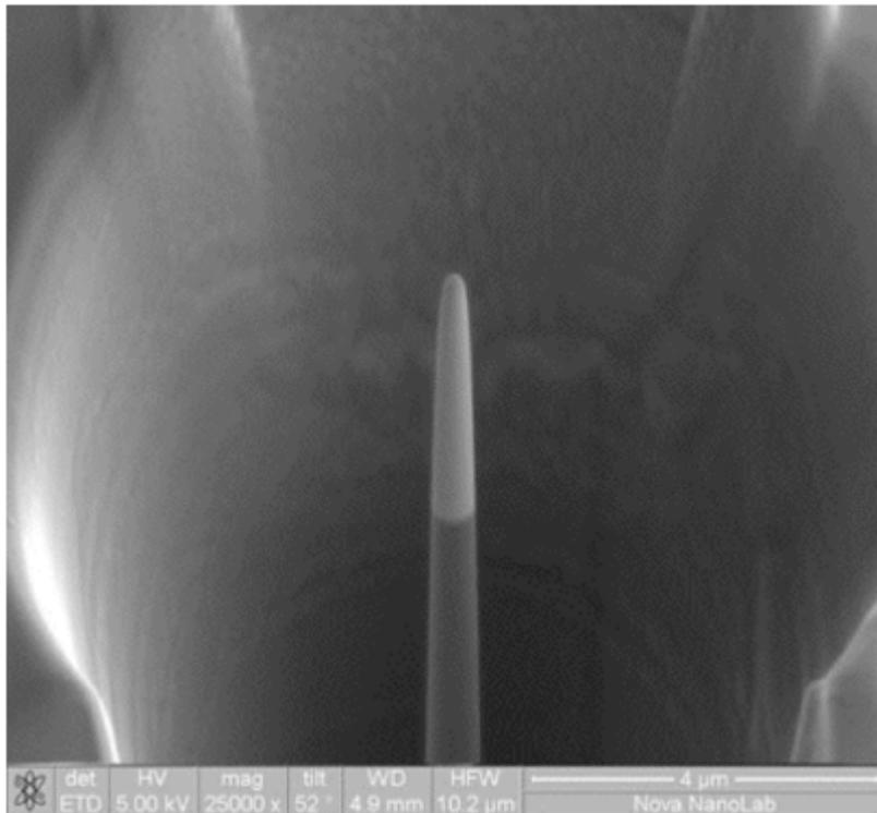
Figure 3: SEM of a needle-like structure measuring about 100 nm at the tip fabricated using FIB tool technology.
