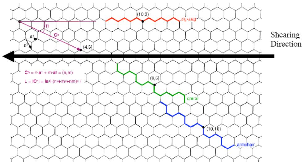
Figure 1: Plan view of graphene sheet material illustrating the direction of the shearing process (x direction) to break carbon to carbon bonds in the material.
