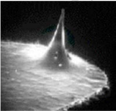
Figure 6: SEM photo of an AFM tip with an extremely sharp tip of less than 40 nm. Another method of making the shearing tools for the mechanosynthesis process is as follows. Starting with a suitable substrate, i.e., silicon, we successively deposit
