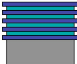
Cored out section of substrate after isotropically etching substrate and one of the thin film materials to create an overhang.
