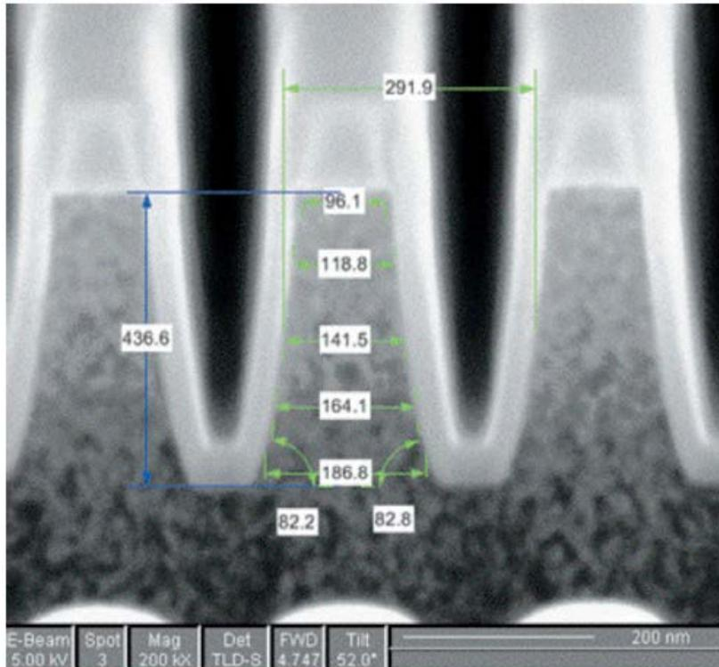
Figure 2: SEM image taken in FIB tool after cross-sectioning (cutting) process. The image scale is 200 nm and the smallest features are 82 nm. The image is displaying the trench isolation of a nanoelectronic device.
