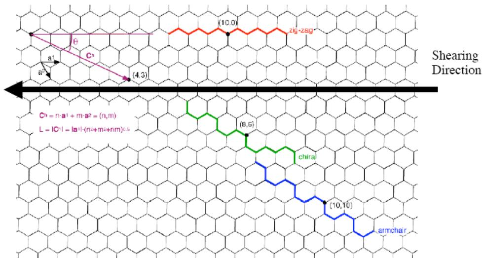
Figure 1: Plan view of graphene sheet material illustrating the direction of the shearing process (x direction) to break carbon to carbon bonds in the material.
