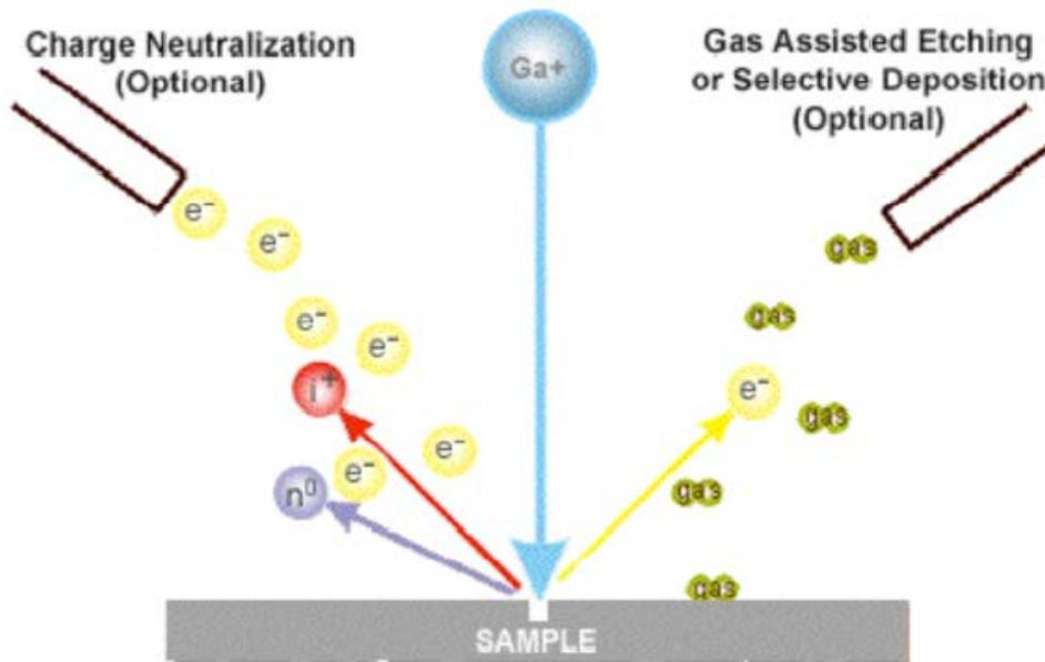
Figure 1: Diagram of the FIB process.
