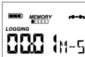
**Image4:** Screen display when switch closed for 1 second
