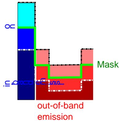
Figure 12. The in-band and out-of-band emission and the waveform mask for swept range emulation. The same losses apply to both in-band and out-of-band emissions.
