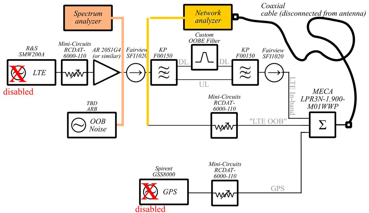
Figure 15. Conducted measurement setup for calibrating LTE out-of-band signal generation
