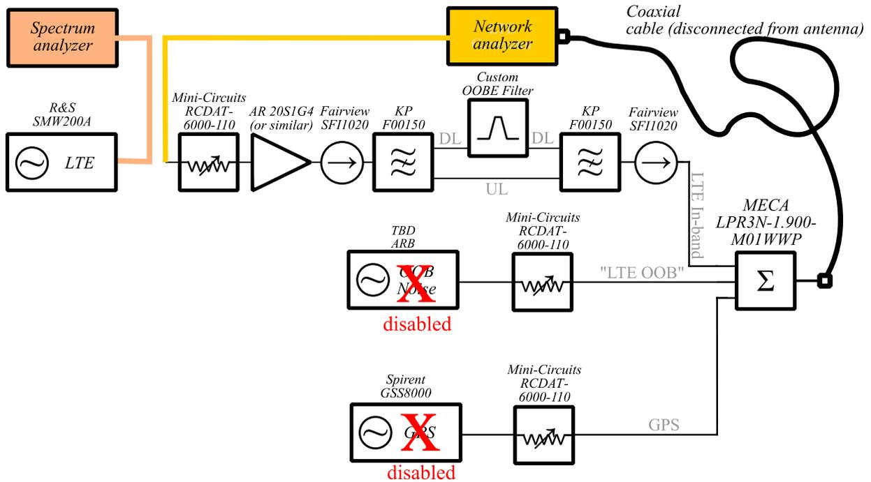
Figure 14. LTE in-band signal generation path conducted measurements for calibrations
