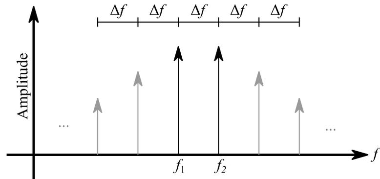
Figure 19. Center frequencies of intermodulation products
