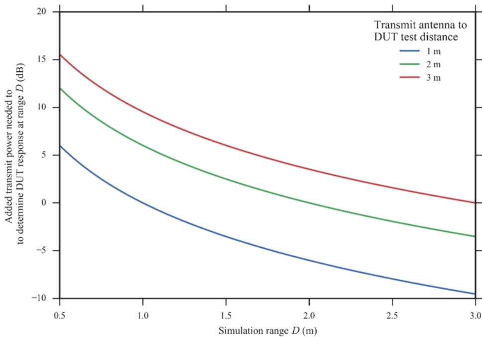
Figure 8. Path loss calculations based on the Friis transmission equation.
