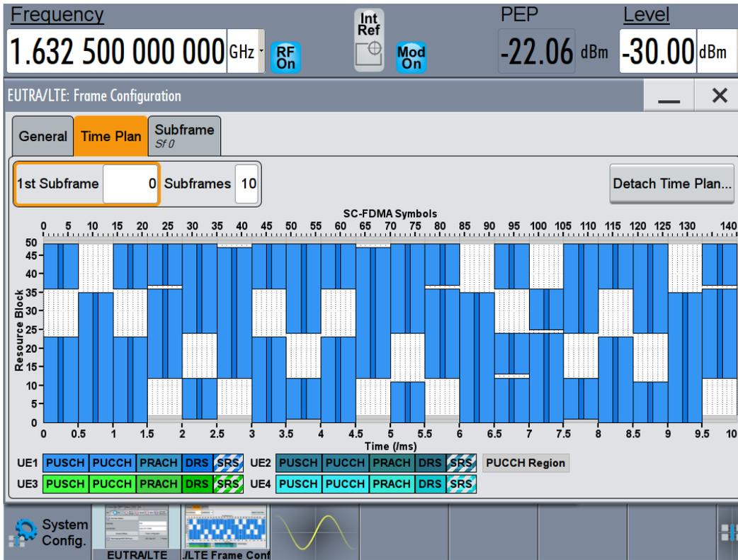
Figure 6. Example LTE uplink resource block allocation
