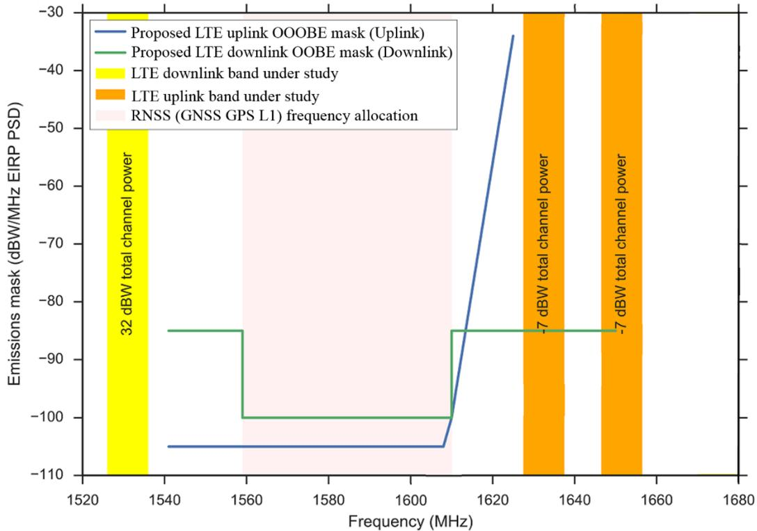
Figure 3. Proposed in-band and out-of-band LTE emission masks under study near the radio navigation satellite service (RNSS) allocation used by GPS L1.
