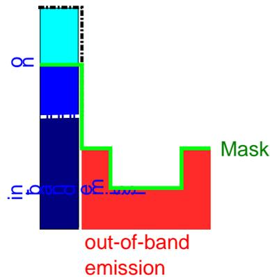
Figure 11. The in-band and out-of-band emission and the waveform mask for in-band LTE coexistence margin testing. Here, LTE out-of-band emission is held constant while LTE in-band emission is varied.
