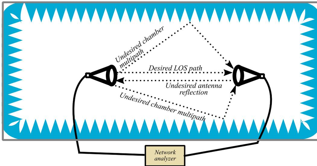
(a) Calibration antenna field uniformity check setup
