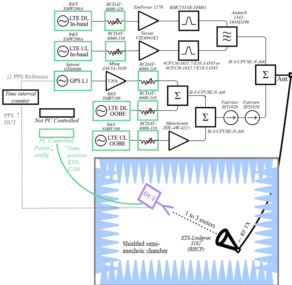
Figure 5 Setup for precision timing tests in the anechoic or semi-anechoic chamber.
