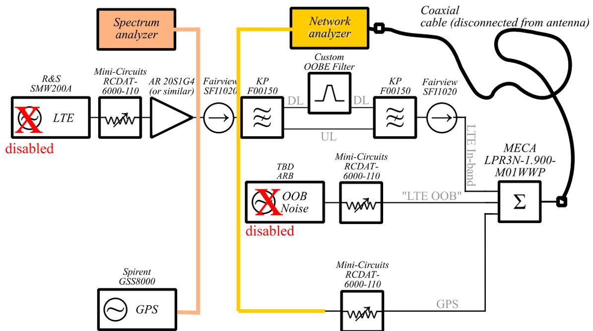
Figure 16. GPS L1 signal generation path conducted measurements for calibrations
