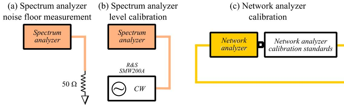
Figure 13. Instrument calibration signal paths
