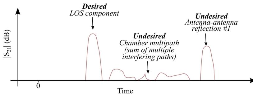
(b) Example field uniformity check by checking power levels in transformed "thru" measurements
