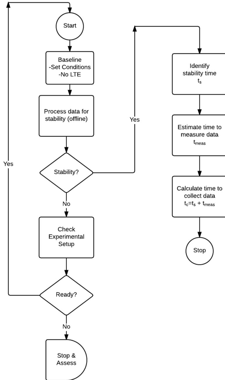
Figure 9. Process to establish data collection time for the DUT.
