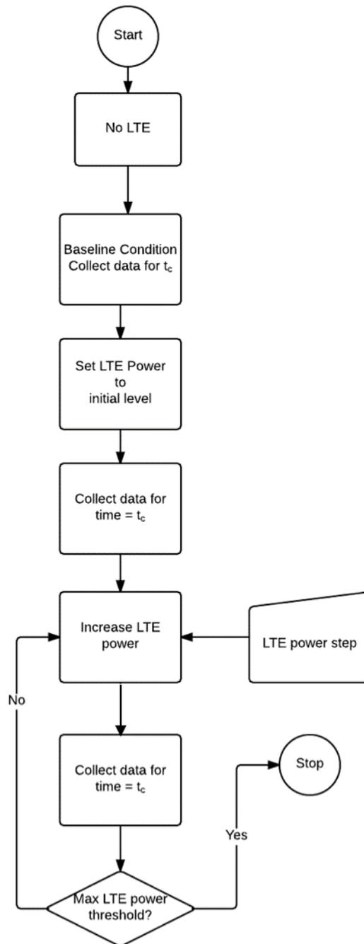
Figure 10. Process to increment LTE power for a specific waveform and collect data from the DUT.
