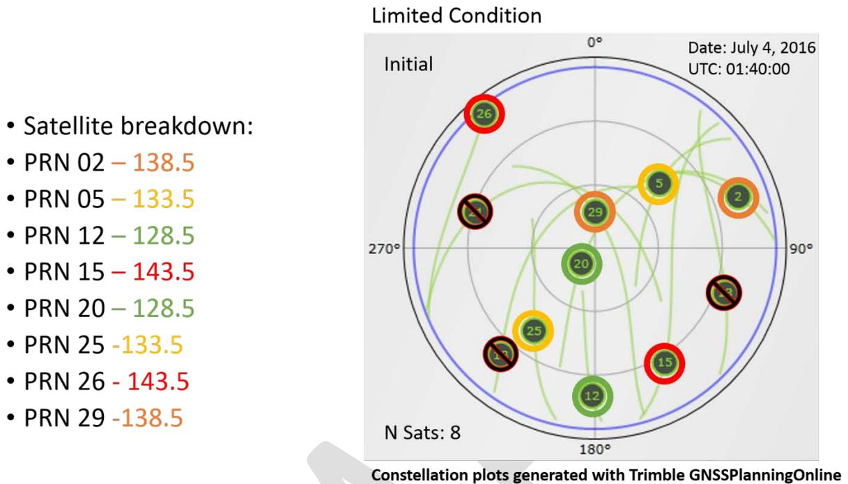
Figure 2. Limited satellite constellation. Initial GPS constellation (left), after 30 mins (right). Satellites in view will have a distribution of power levels at the plane of the receiver assuming a 0 dBi receiving antenna.
