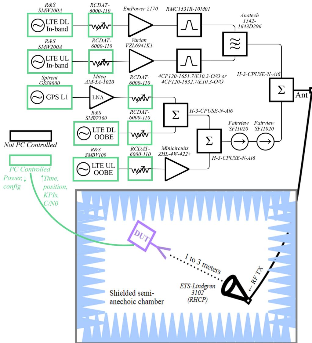
Figure 4. Setup for position measurements in the anechoic or semi-anechoic chamber.
