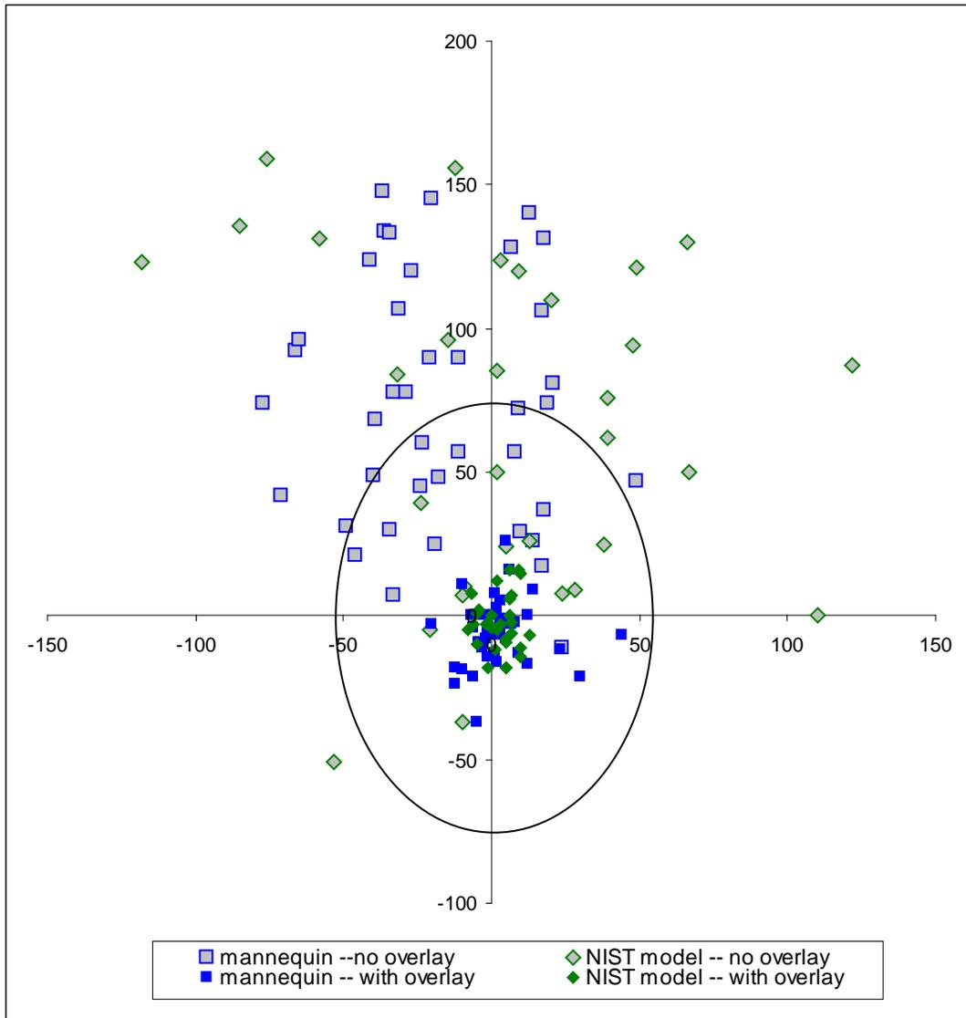
Figure 7: Displacement of image center from target center
