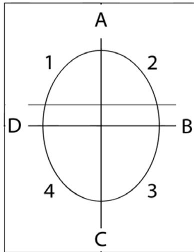
**Figure 4: Positions for Measuring Face Placement**
