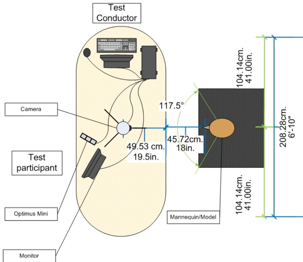
**Figure 2: Face overlay test layout**
