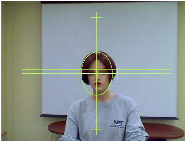
**Figure 3: Use of the overlay to frame the face in the image**
