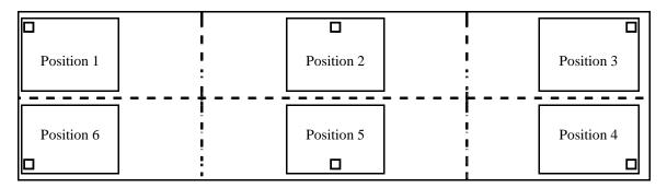
$\Box = \text{Load Bearing Point}$ (Added 2003)
