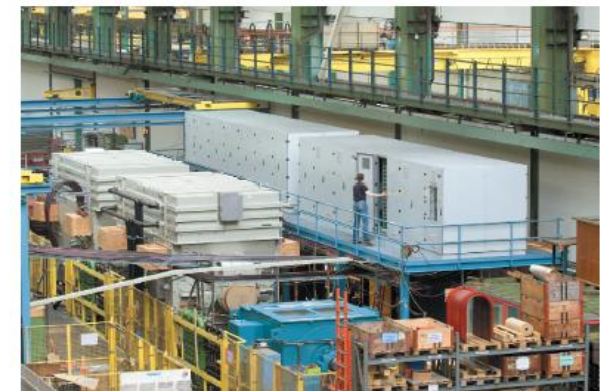
Back-to-back test 48 MW / 3,500 rpm
