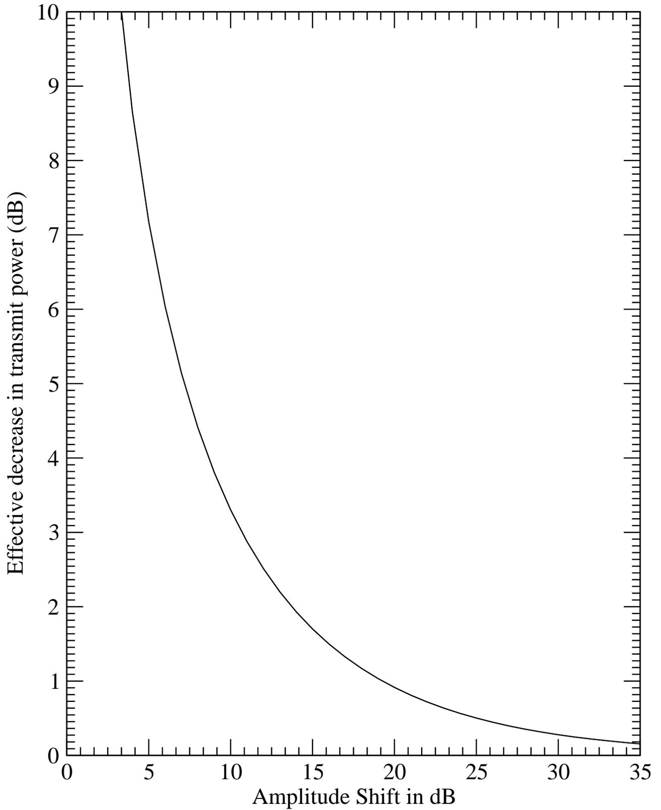
Figure 2: The equivalent loss in signal level when an amplitude shift of  $X$ dB is used instead of on-off keying for binary ASK modulation.
