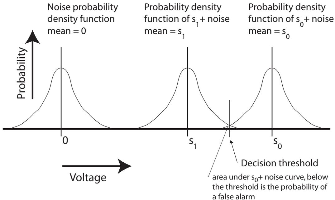
Figure 1: Diagram of voltages used to determine which ASK bit was sent.
