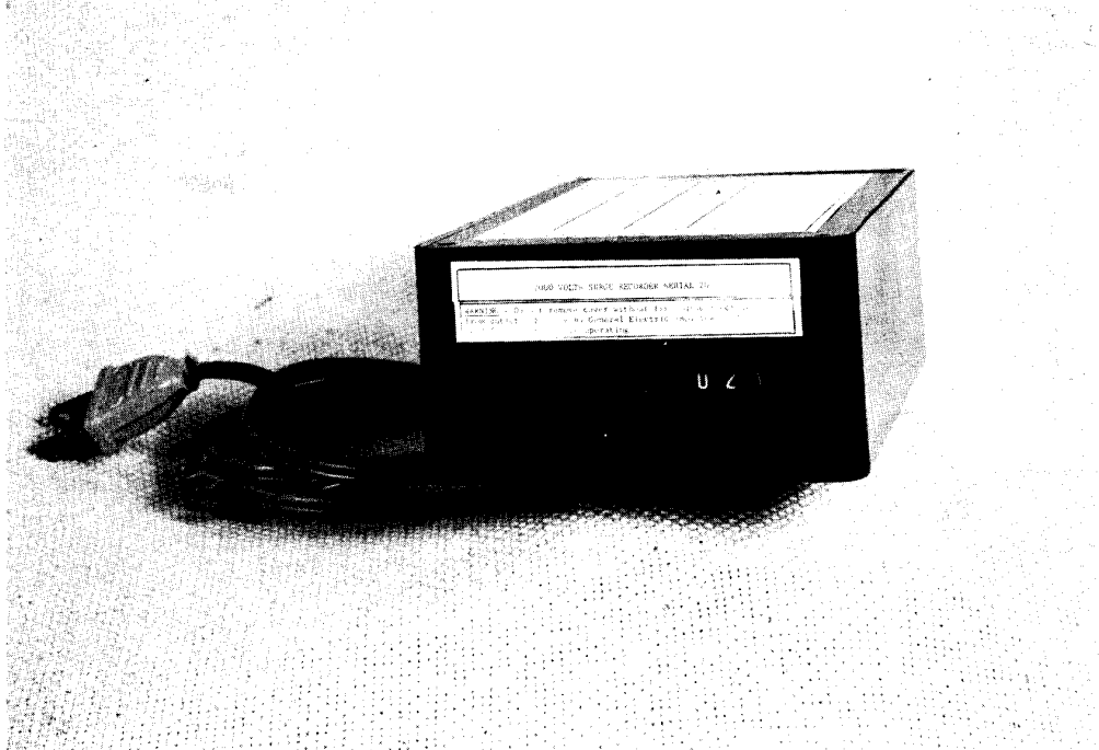
Surge counter - connecting cord is only accessible part, with non-reset counter behind window.
