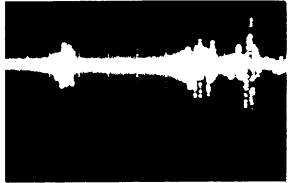
Figure 4. Transients induced by lightning in overhead data cable Vertical: 4 V/div Sweep: 1 ms/div Cable: 1000 m long, 5 m high (courtesy Digital Equipment Corporation)
