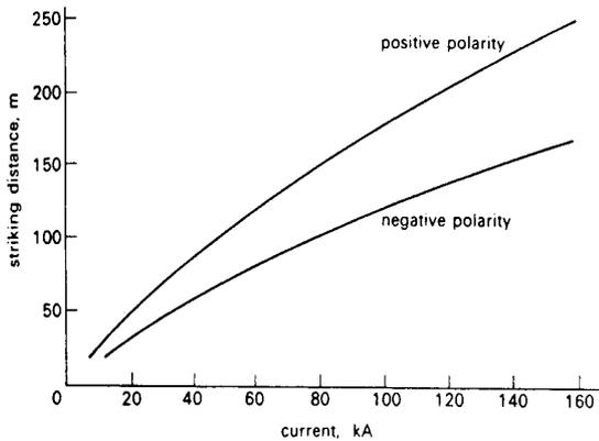
Figure 3-4. Relationship between potential current level of return stroke and striking distance
