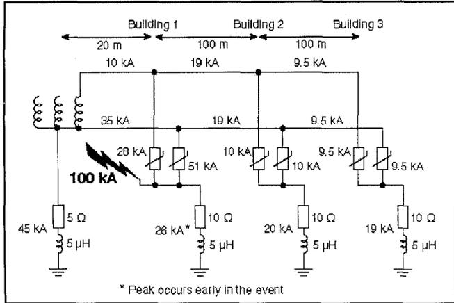
Figure 9 - Daisy chain TT 2-wire configuration with building next to distribution transformer struck by a 10/350 μs, 100 kA surge
