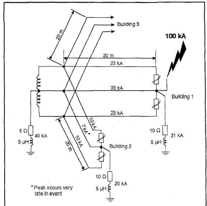
Figure 3 - Radial TN configuration with three buildings supplied by one distribution transformer, one building struck by a 10/350  $\mu$ s, 100 kA surge, showing peak values of currents shared among available paths.
