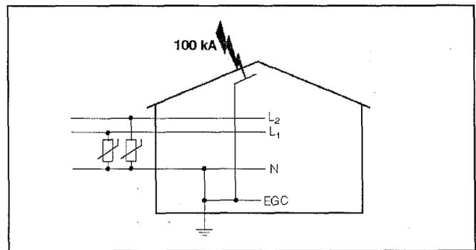
Figure 1. Service connections in a 3-wire TN system
