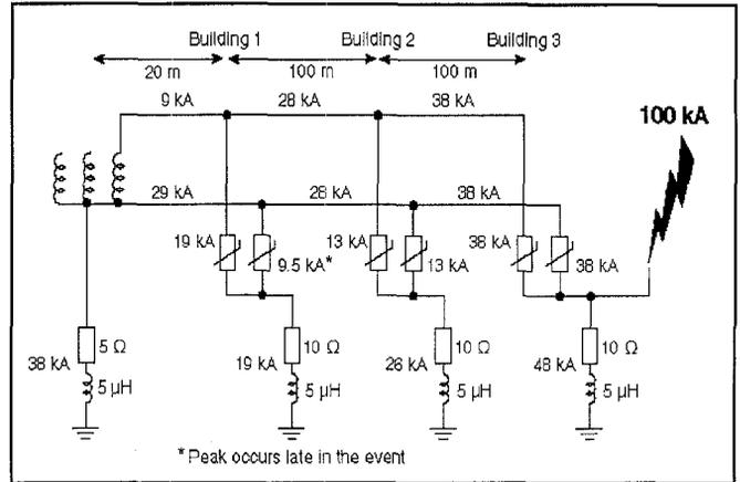
Figure 11 - Daisy chain TT 2-wire configuration with building at opposite end of distribution transformer struck by a 10/350 μs, 100 kA surge
