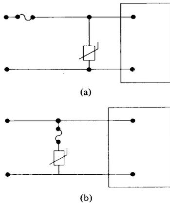
Fig. 6. Options for varistor fuse connection. (a) Protection maintained, function interrupted. (b) Function maintained, protection lost.
