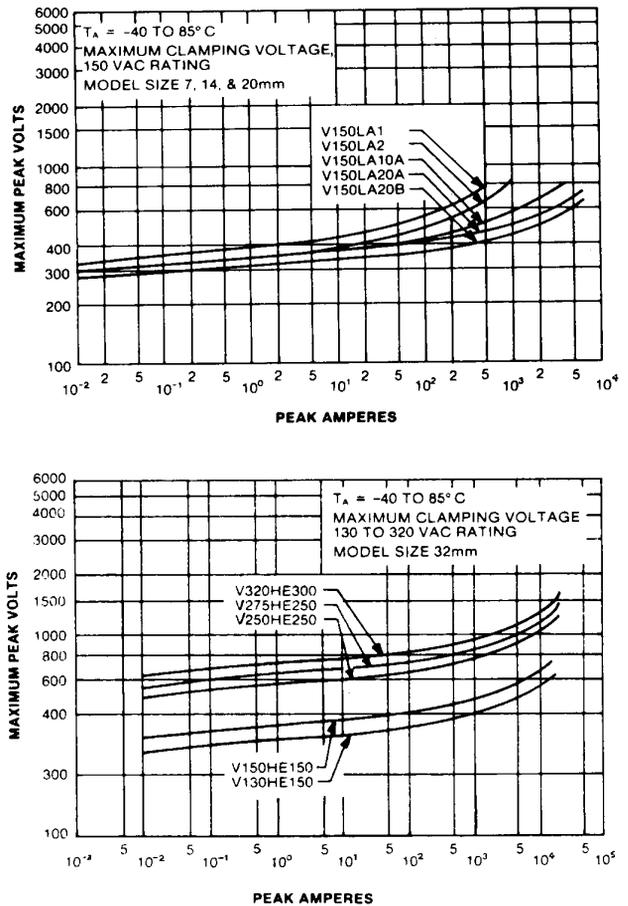
Fig. 4. V-I characteristics for 14-, 20-, and 32-mm varistors rated 150-V rms.
