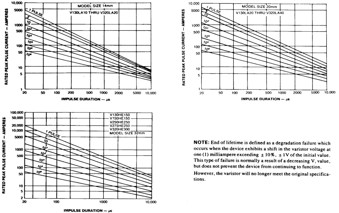
**NOTE:** End of lifetime is defined as a degradation failure which occurs when the device exhibits a shift in the varistor voltage at one (1) milliampere exceeding  $\pm 10\%$ ,  $\pm 1V$  of the initial value. This type of failure is normally a result of a decreasing  $V_1$  value, but does not prevent the device from continuing to function. However, the varistor will no longer meet the original specifications.
