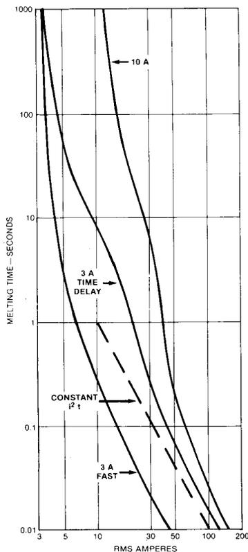
Fig. 8. Time-current characteristic of fast fuse and of time-delay fuse.
