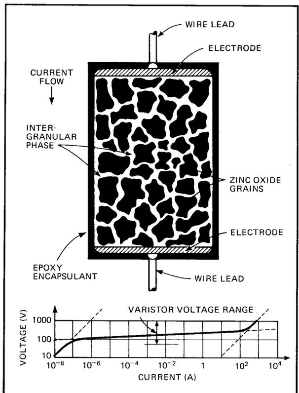
**1. Properties.** Two-phase material in body of metal-oxide-type varistor acts as insulator for low applied voltages and as conductor for transients that exceed device's clamping voltage. Bistable intergranular phase containing bismuth oxide surrounds each conductive zinc oxide grain. Idealized V-I curve illustrates unit's nonlinear behavior in varistor voltage range.
