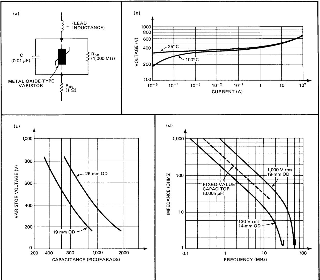
one with a 130-v rms rating, and the other with a 1,000-v rms rating. A point-of-reference curve for a fixed 0.005-microfarad capacitor is also included.
