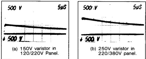
Figure 16: Clamping voltage of varistors with short leads
