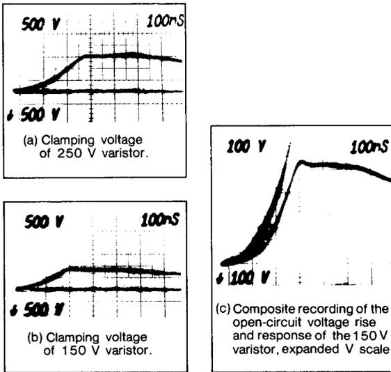
Figure 7: Clamping voltage of metal oxide varistors
