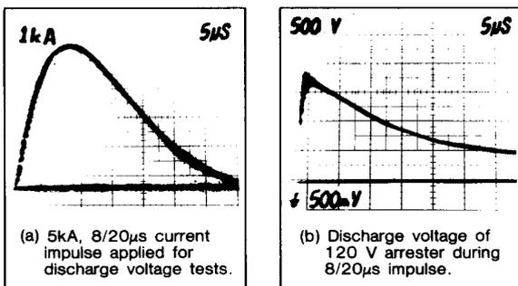
Figure 11: Applied impulse and 120 V arrester response
