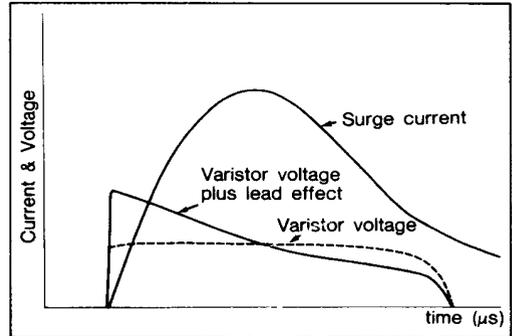
Figure 5: Degradation of clamping voltage caused by misapplication
