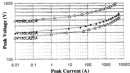
Fig. 1. MOV characteristics obtained from modeling results.
