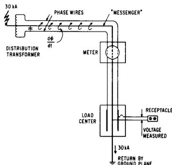
Fig. 9. Voltages induced in the house wiring system.
