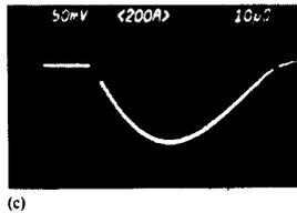
current on the varistor. (The current in the suppressor is lower than the available short-circuit current as a result of the reduced driving voltage, because the varistor holds off 600 V.
