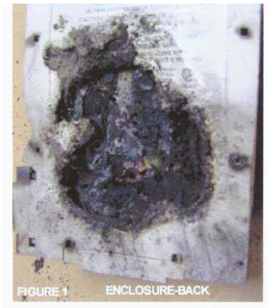
Figure 3 – Field failure submitted for assessment (Courtesy U.S. Consumer Product Safety Commission)
