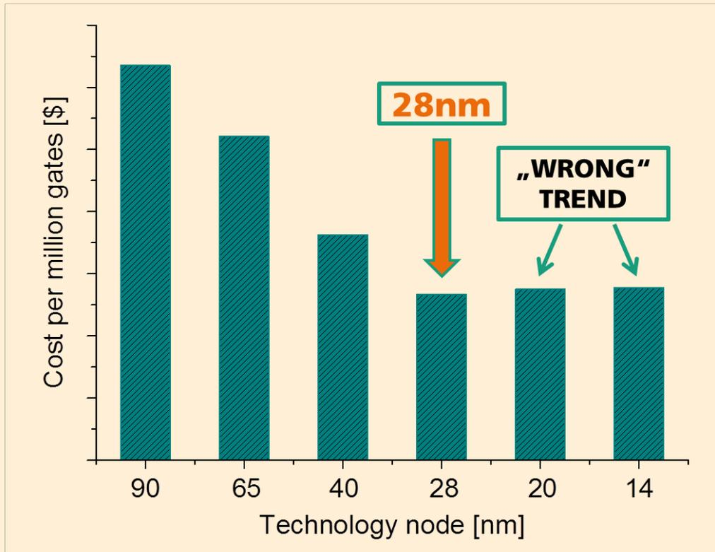
No cost /transistor crossover for the first time at the transition from 28nm → 20nm node
