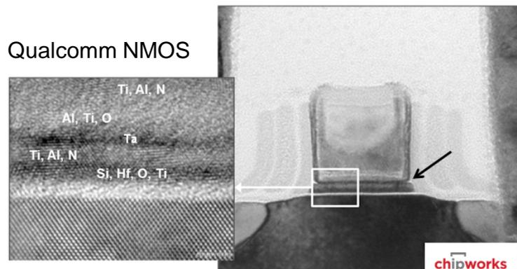
Figure 1 NMOS Transistor in Qualcomm Snapdragon 800
