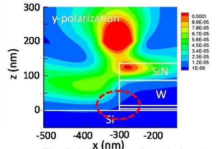
Excitation light intensity distribution modified by sample structure → Significant impact on Raman spectra
