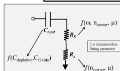
Fig. 10 Simple circuit model of the tip-sample interaction in the junction between the SMM sample and the Si dopant profile sample.
