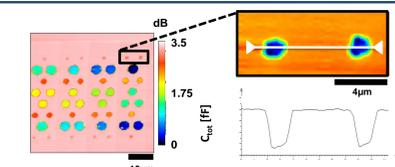
Fig. 14 SMM image of calibration sample with detail and cross-section.
