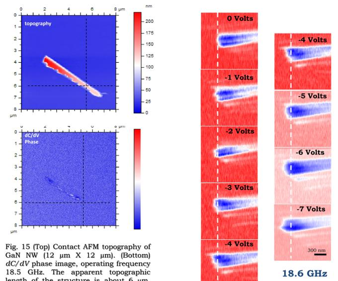
Fig. 15 (Top) Contact AFM topography of GaN NW (12 μm X 12 μm). (Bottom) dC/dV phase image, operating frequency 18.5 GHz. The apparent topographic length of the structure is about 6 μm. However, the apparent length decreases to about 4 μm in simultaneously acquired dC/dV amplitude and phase images (phase image shown). In other words, only the n-type segment of the NW shows a response in the dC/dV images.
