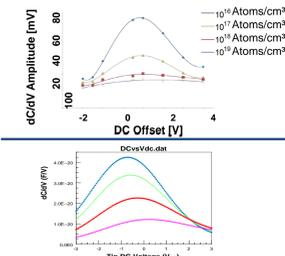
Fig. 6 Comparison of measurement (top) to simulation (bottom) used to extract calibration parameters with NIST FastC2D [3].
