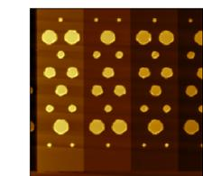
Fig. 12 AFM topography of calibration samples for absolute capacitance calibration.
