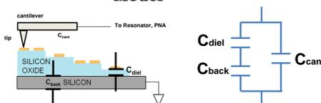
Fig. 13 Circuit model for absolute capacitance calibration.
