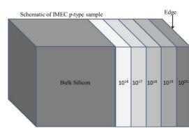
Fig. 4 Calibration samples for dopant profiling.
