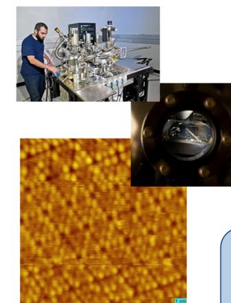
Fig. 17 Image of Si(111) 7x7 surface taken with new multi-probe system.
