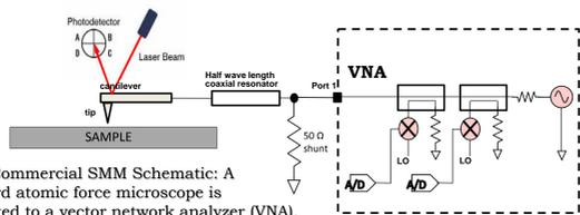
Fig. 1 Commercial SMM Schematic: A standard atomic force microscope is connected to a vector network analyzer (VNA). A conductive cantilever tip is used for transmitting an incident microwave signal to the sample.
