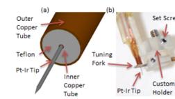
Fig. 2 (a) Schematic of probe tip construction (b) Photo of tuning fork holder
