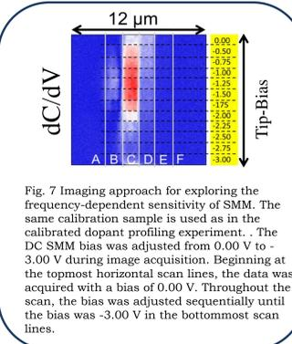
Fig. 7 Imaging approach for exploring the frequency-dependent sensitivity of SMM. The same calibration sample is used as in the calibrated dopant profiling experiment. The DC SMM bias was adjusted from 0.00 V to -3.00 V during image acquisition. Beginning at the topmost horizontal scan lines, the data was acquired with a bias of 0.00 V. Throughout the scan, the bias was adjusted sequentially until the bias was -3.00 V in the bottommost scan lines.
