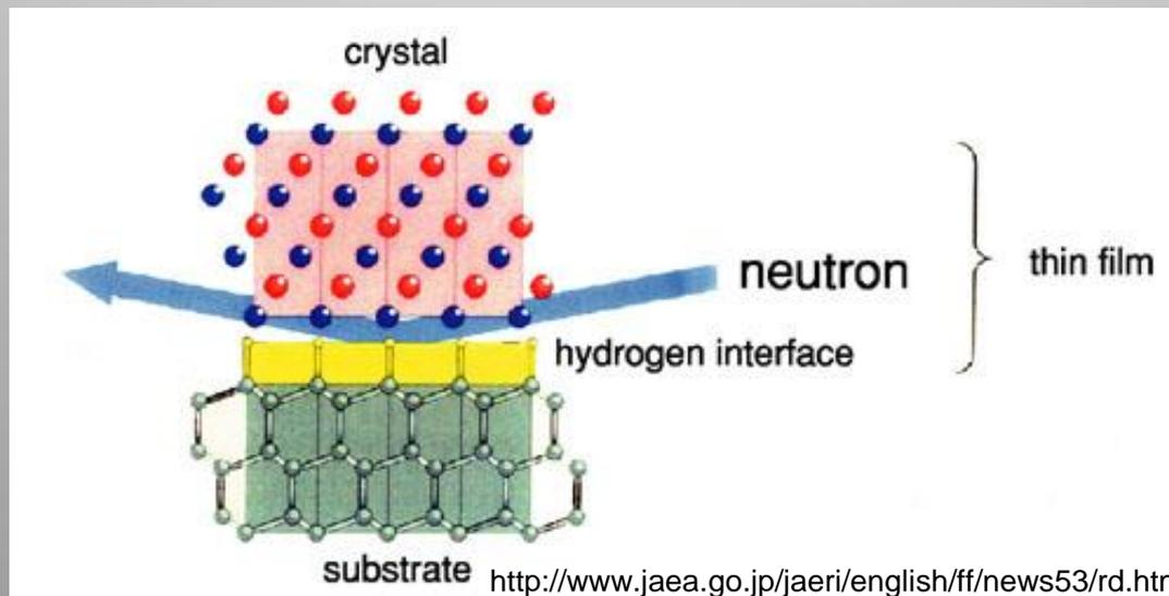
**Hydrogen interface characterized by using neutron reflectometry**
