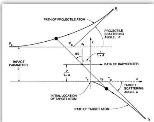
In principle, MD simulates the physical movement of atoms and molecules in the context of multi-body effects, whereas in BCA, the ion is approximated to travel through a material by experiencing a sequence of independent binary collisions with sample atoms. A large simulation volume has to be considered for FIB simulation. Therefore a BCA code named TRIDYN is used in this study.
