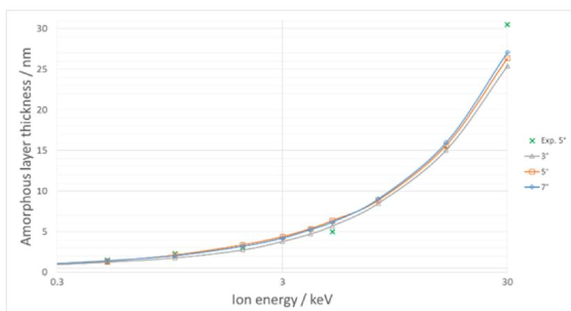
1. TRIDYN Simulated amorphous Si layer thickness as a function of ion energy for 3°, 5° and 7° ion impingement angle. Experimental TEM data are also depicted for comparison.
