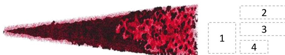
3 & 4. APT determined Ga concentration profiles from three APT samples, with corresponding TRIDYN simulation (3); illustration of APT measurement (Ga: black and Si: red) (4).
