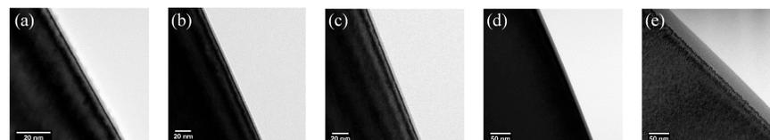
2. TEM images of a c-Si cross-section after a 0.5/1/2/5/30kV Ga FIB process show amorphous layer thicknesses of 1.5/2.3/3.1/5.0/30.5nm, from (a) to (e) respectively.
