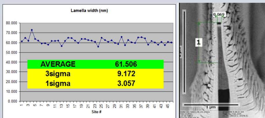
Figure 1. Thickness consistency of TEM samples prepared via automated FIB
