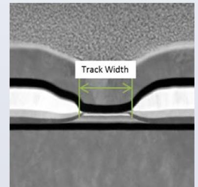
Figure 3. STEM image showing strong material contrast of a GMR reader
