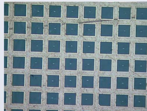
Figure 2. TEM grid with multiple samples
