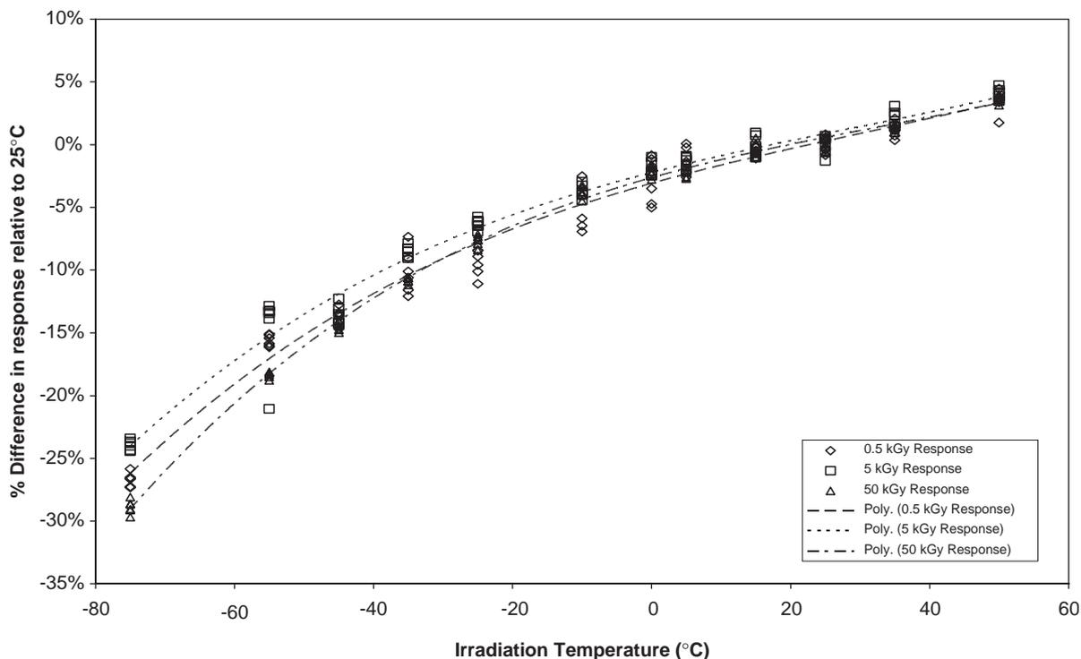
Fig. 4. Relative dose response of Harwell alanine dosimeters irradiated to absorbed doses of 0.5, 5 and 50 kGy at fixed temperatures ranging from  $-77^{\circ}\text{C}$  to  $-10^{\circ}\text{C}$  (measured at NIST).
