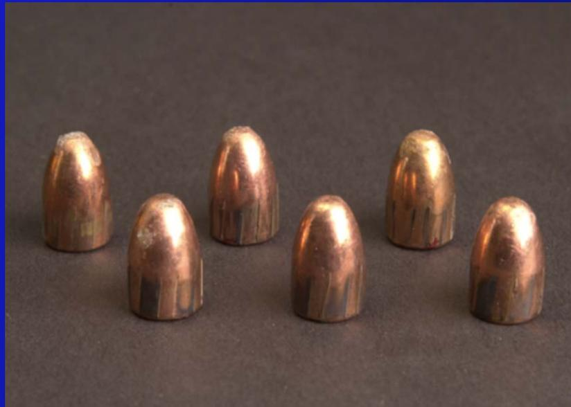
Six master bullets used for topography measurements
