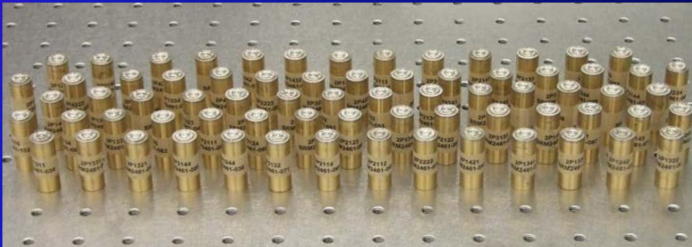
SRM Casings made from electroform process
