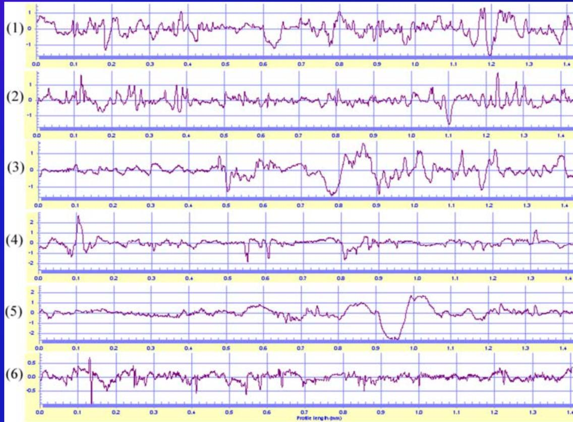
Surface Profile measurements from the six lands on the Standard Bullet
