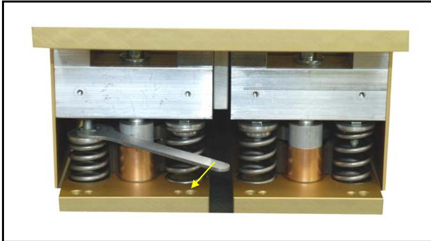
If an adjustment is needed turn the M6 nuts using the spanner provided. Adjust all springs on both sides equally. Moving the spanner to the left raises the units.
