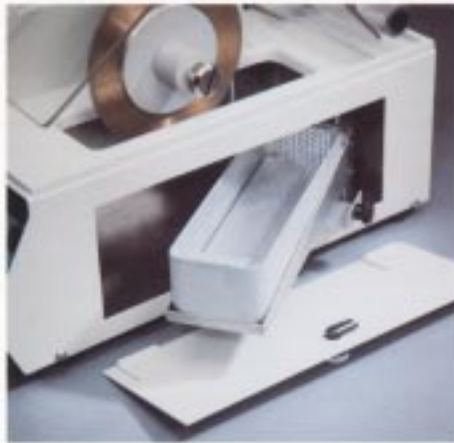
Sectioned samples are easily retrieved through the side coolant tray door and basket.
