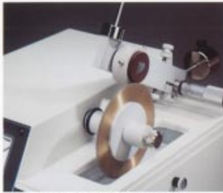
Mounted samples can be sectioned effectively with proper selection of chucks and flanges.
