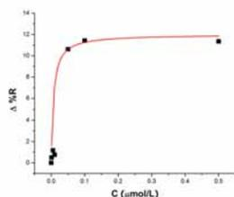
Binding curves for quantum dots adsorption to collagen layer in the microchannels
