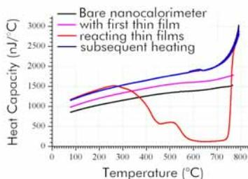
Nanocalorimeter data showing the reaction between nanometer scaled silicon and nickel thin films to form nickel silicide.
