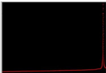
Nanocalorimeter data showing a sharp melting peak achieved from a 50 nm thin film of pure aluminum. The sample mass is  $\approx 400$  ng.
