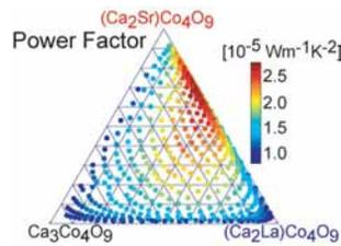
Power factor of La and Sr substituted Ca<sub>3</sub>Co<sub>4</sub>O<sub>9</sub> thermoelectric materials
