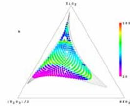
Dielectric constants of HfO<sub>2</sub>-TiO<sub>2</sub>-Y<sub>2</sub>O<sub>3</sub> alloys
