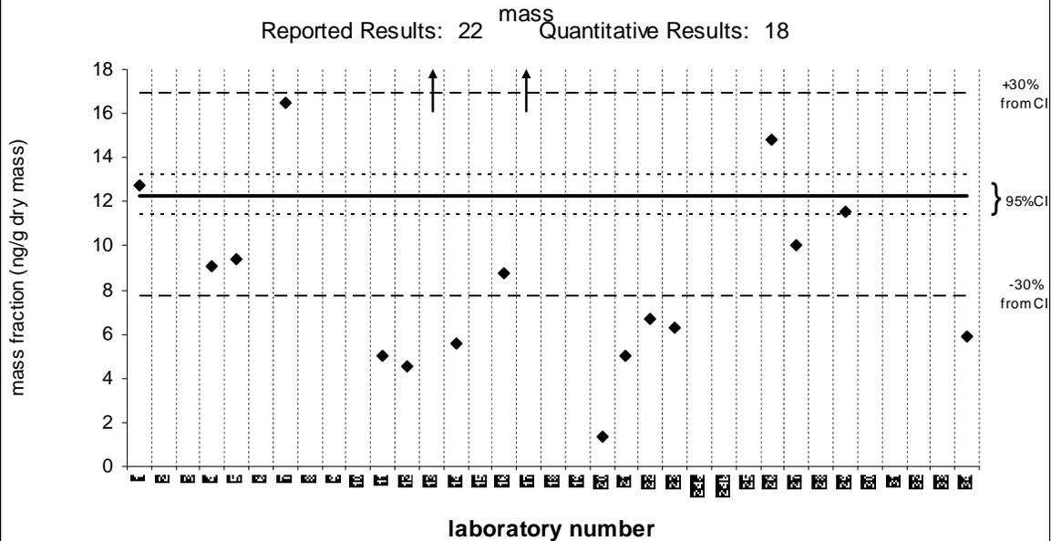
Solid line: value from Certificate of Analysis ; dotted line: 95% confidence limits; dashed line: 30% from 95% confidence limits
