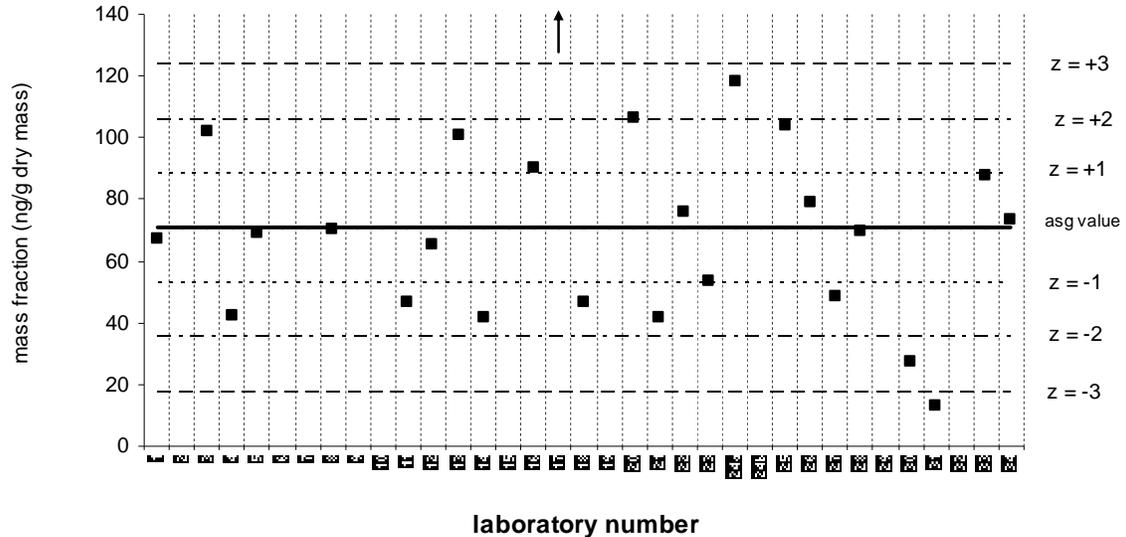
Solid line : exercise assigned value (EAV); dotted line:  $z = \pm 1$  (25% from EAV); dotted/dashed line:  $z = \pm 2$  (50% from EAV); dashed line:  $z = \pm 3$  (75% from EAV)
