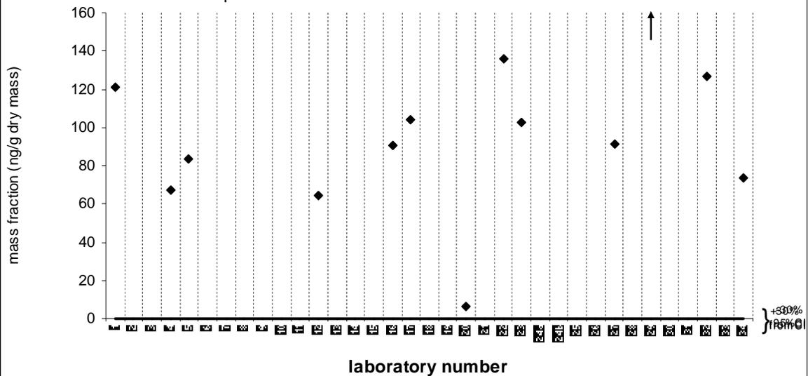
Solid line: value from Certificate of Analysis ; dotted line: 95% confidence limits; dashed line: 30% from 95% confidence limits
