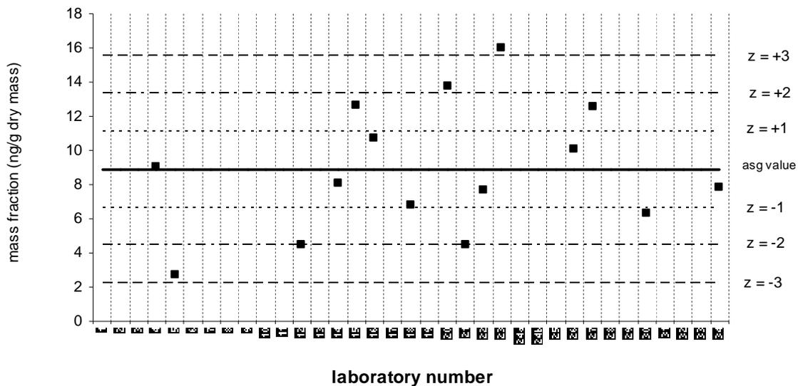
Solid line : exercise assigned value (EAV); dotted line:  $z = \pm 1$  (25% from EAV); dotted/dashed line:  $z = \pm 2$  (50% from EAV); dashed line:  $z = \pm 3$  (75% from EAV)
