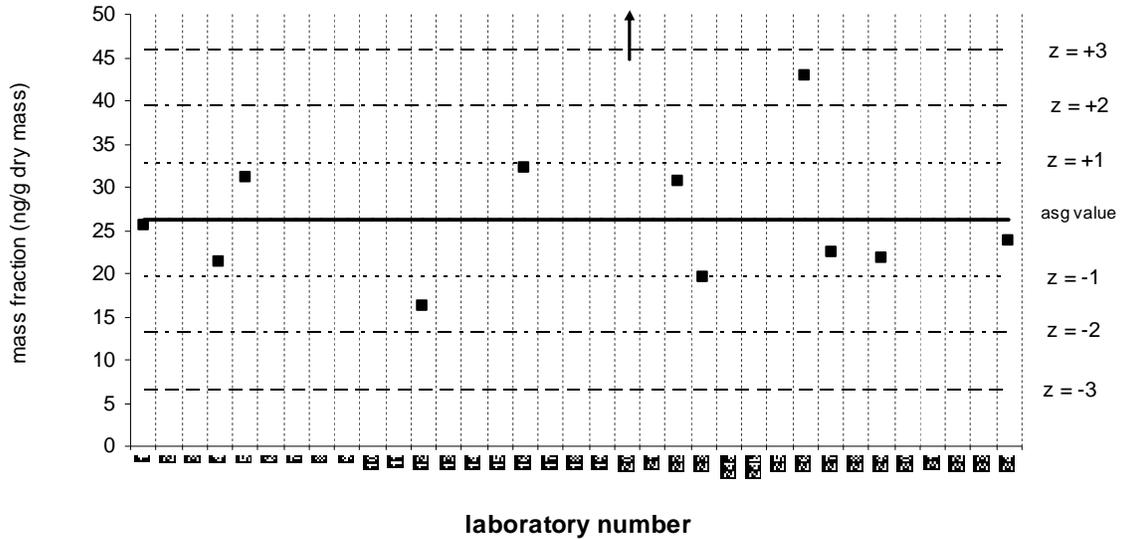
Solid line : exercise assigned value (EAV); dotted line: z=±1 (25% from EAV); dotted/dashed line: z=±2 (50% from EAV); dashed line: z=±3 (75% from EAV)
