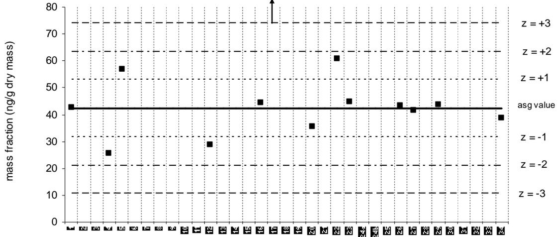
Solid line : exercise assigned value (EAV); dotted line: z=±1 (25% from EAV); dotted/dashed line: z=±2 (50% from EAV); dashed line: z=±3 (75% from EAV)
