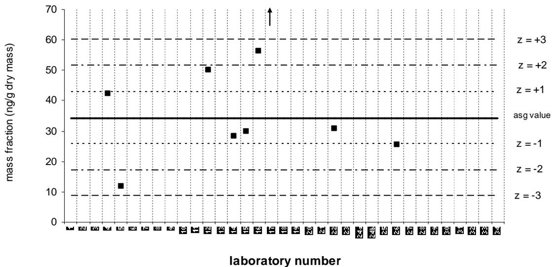
Solid line : exercise assigned value (EAV); dotted line: z=±1 (25% from EAV); dotted/dashed line: z=±2 (50% from EAV); dashed line: z=±3 (75% from EAV)
