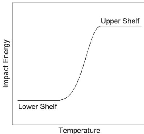
*Figure 1. A temperature transition curve.*
