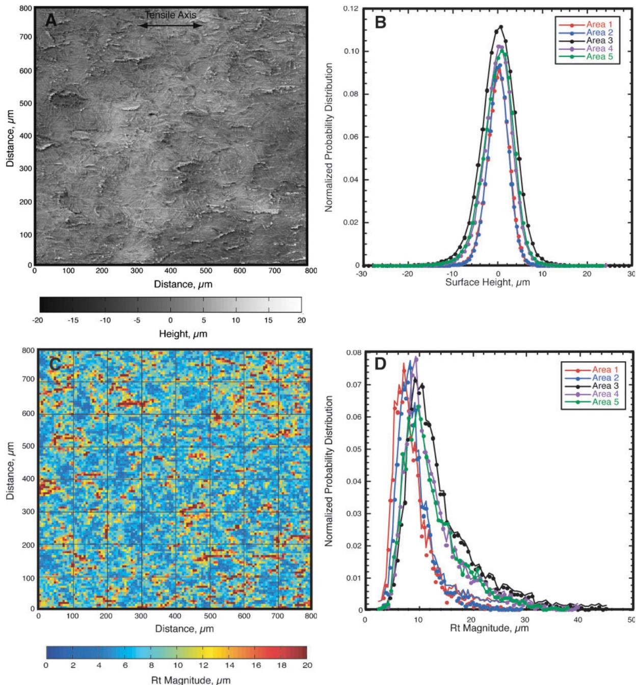
A topography of AA 5754-O at maximum uniform strain condition in uniaxial strain mode; B corresponding distribution of surface heights for each of five areas sampled in this strain condition; C Rt map constructed from topography shown in A; D corresponding distribution of Rt values for each of five Rt maps
