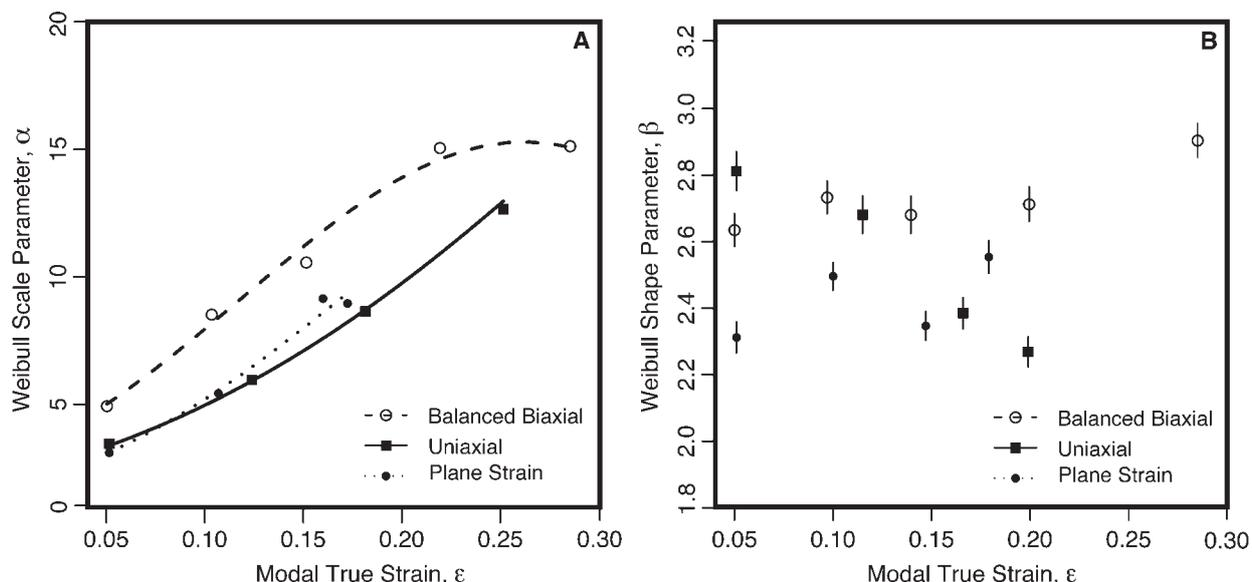
A Weibull scale parameter  $\alpha$  as function of modal true strain; B Weibull shape parameter  $\beta$  as function of modal true strain
