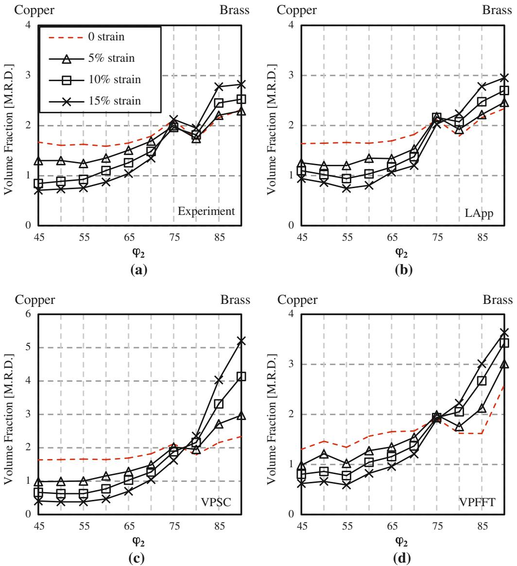
Fig. 18— $\beta$ -fiber volume fraction plots for the TD-oriented plane strain from (a) the experiment, (b) the LApp simulation, (c) the VPSC simulation, and (d) the VPFFT simulation. Note the scale change in (c) the VPSC plot.
