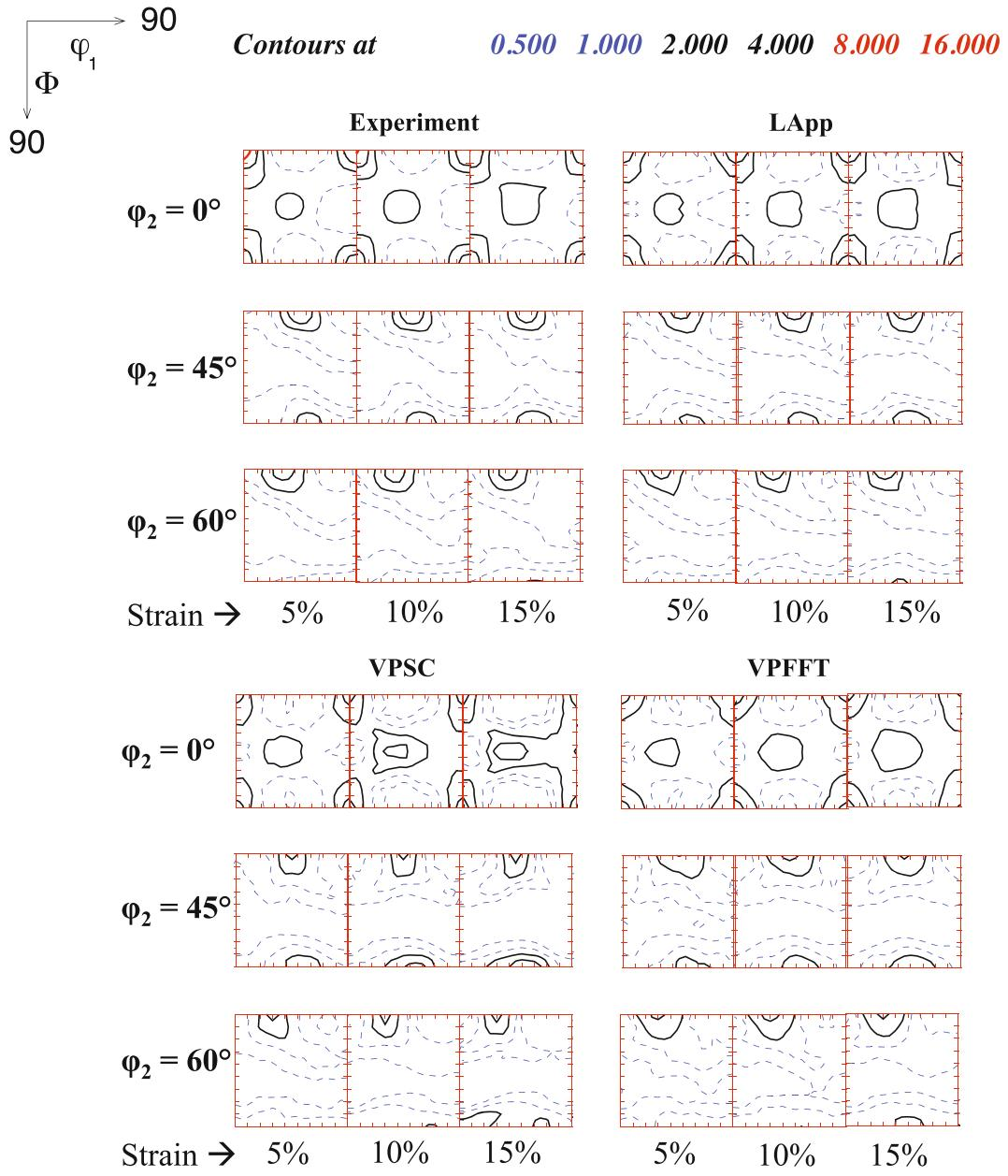
Fig. 13—Comparison of OD sections for TD-oriented plane strain tension. The strain levels are 5, 10, and 15 pct in TD.
