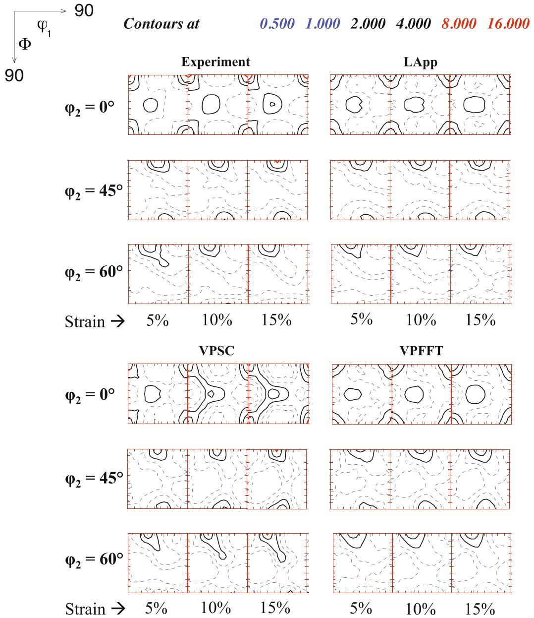
Fig. 11—Comparison of OD sections for TD uniaxial tension. The strain levels are 5, 10, and 15 pct in TD.
