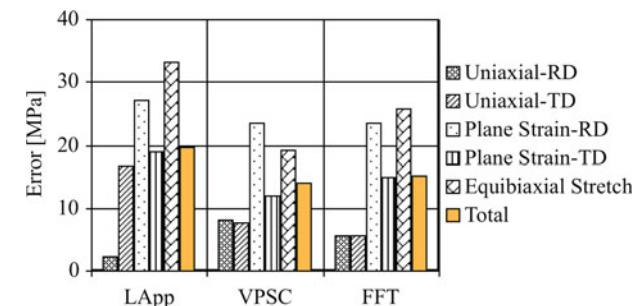
Fig. 9—Bar chart for the quality of fit to the experimental data in the five strain paths for the three different viscoplasticity models. The error value in the vertical axis is the RMS difference between the simulated stress-strain curves and the experimental data.
