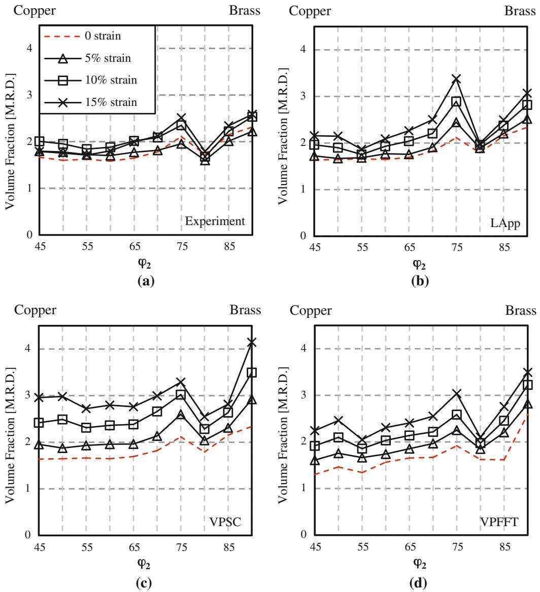
Fig. 17— $\beta$ -fiber volume fraction plots for the RD-oriented plane strain from (a) the experiment, (b) the LApp simulation, (c) the VPSC simulation, and (d) the VPFFT simulation.
