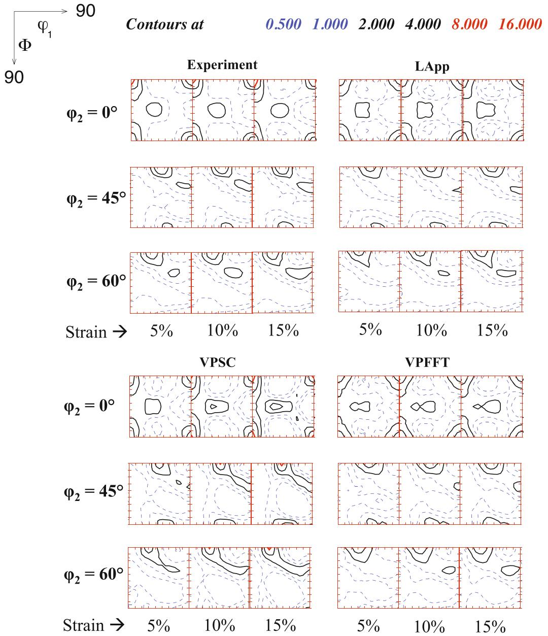
Fig. 10—Comparison of OD sections for RD uniaxial tension. Strain levels are 5, 10, and 15 pct in RD.
