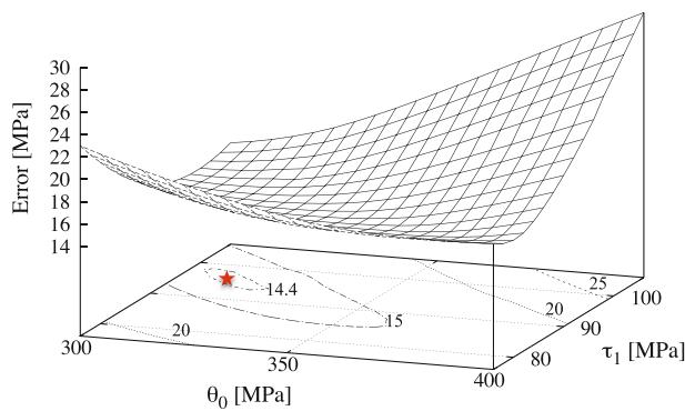
Fig. 3—3-D plot of the error vs the initial hardening rate  $\theta_0$  and CRSS  $\tau_1$ . The error values are projected on the bottom and plotted with contour levels. A single minimum is found at  $\{\theta_0, \tau_1\} = \{310, 96\}$ , noted by the star.
