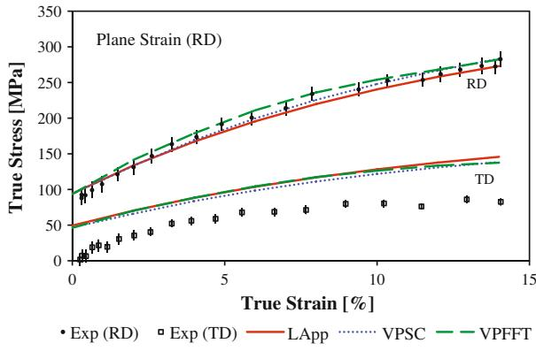
Fig. 6—Comparison of measured and simulated stress-strain curves for RD-oriented plane strain tension. The horizontal axis is the true strain in RD, and stresses both in RD and TD are plotted in the graph.
