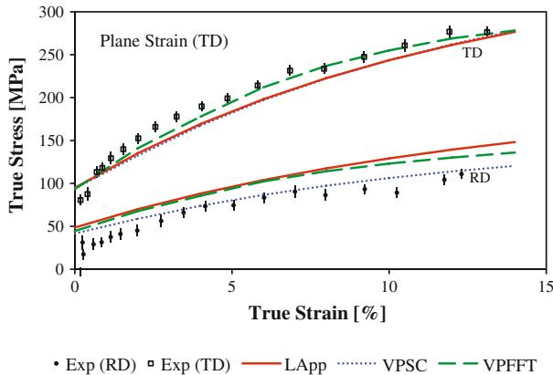
Fig. 7—Comparison of measured and simulated stress-strain curves for TD-oriented plane strain tension. The horizontal axis is the true strain in TD, and stresses both in RD and TD are plotted in the graph.
