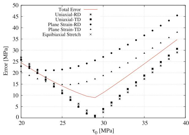
Fig. 2—Error vs the initial CRSS  $\tau_0$ . A single minimum of the total error is found at  $\tau_0 = 29$  MPa.
