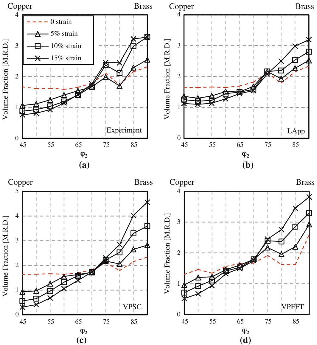
Fig. 16— $\beta$ -fiber volume fraction plots for the TD uniaxial tension from (a) the experiment, (b) the LApp simulation, (c) the VPSC simulation, and (d) the VPFFT simulation.
