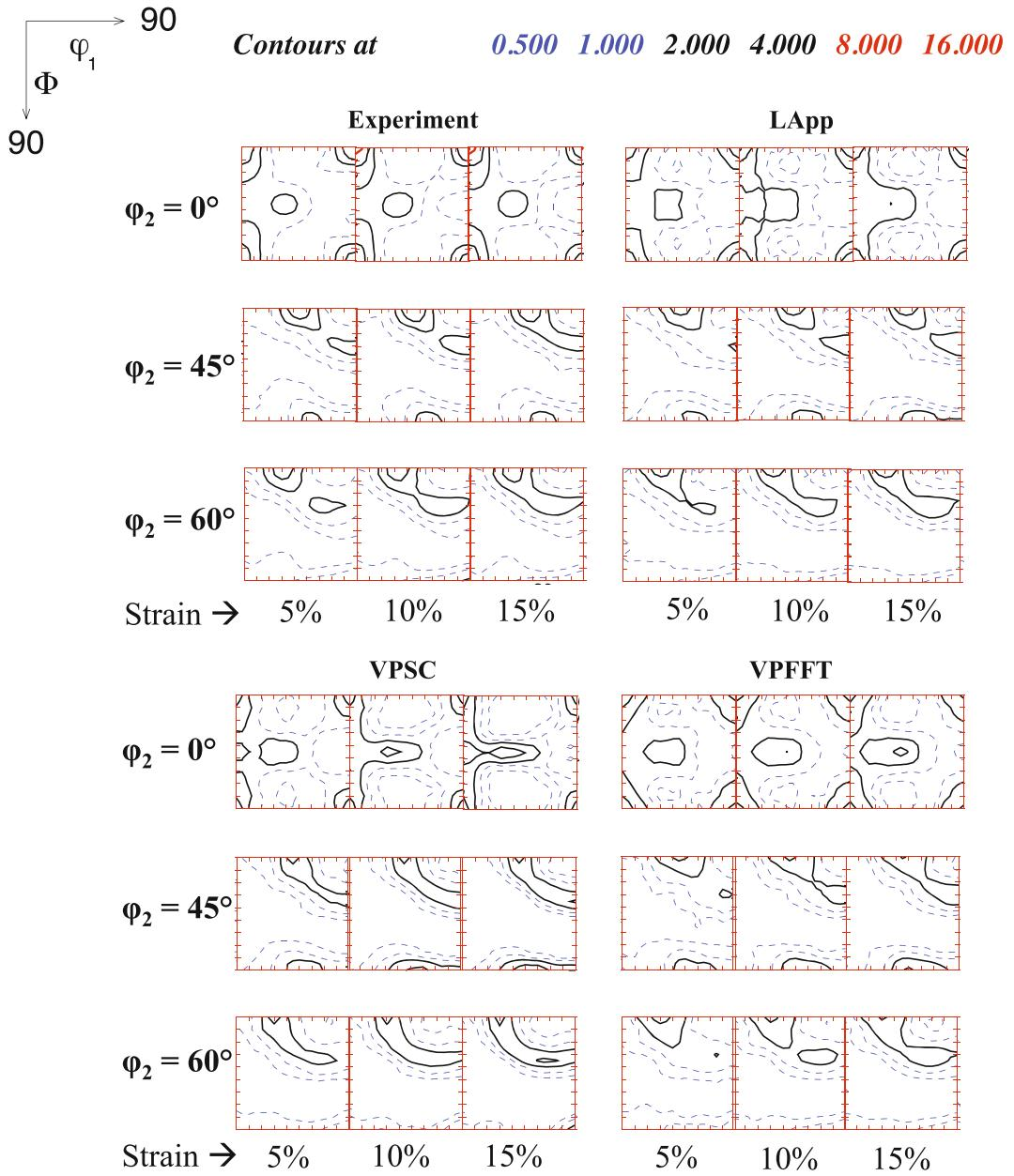
Fig. 12—Comparison of OD sections for RD-oriented plane strain tension. The strain levels are 5, 10, and 15, in RD.
