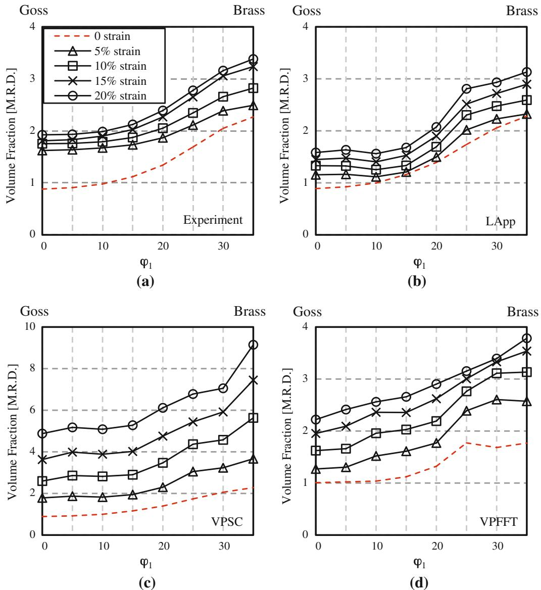
Fig. 19—<110>-fiber ( $\varphi_1 = 0$  to  $35$  deg,  $\Phi = 45$  deg, and  $\varphi_2 = 0$  deg) volume fraction plots for equibiaxial stretch from (a) the experiment, (b) the LApp simulation, (c) the VPSC simulation, and (d) the VPFFT simulation. Note the scale change in (c) the VPSC plot.
