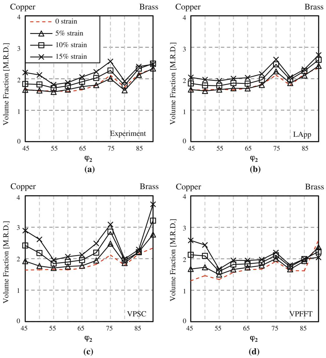
Fig. 15— $\beta$ -fiber volume fraction plots for the RD uniaxial tension from (a) the experiment, (b) the LApp simulation, (c) the VPSC simulation, and (d) the VPFFT simulation.
