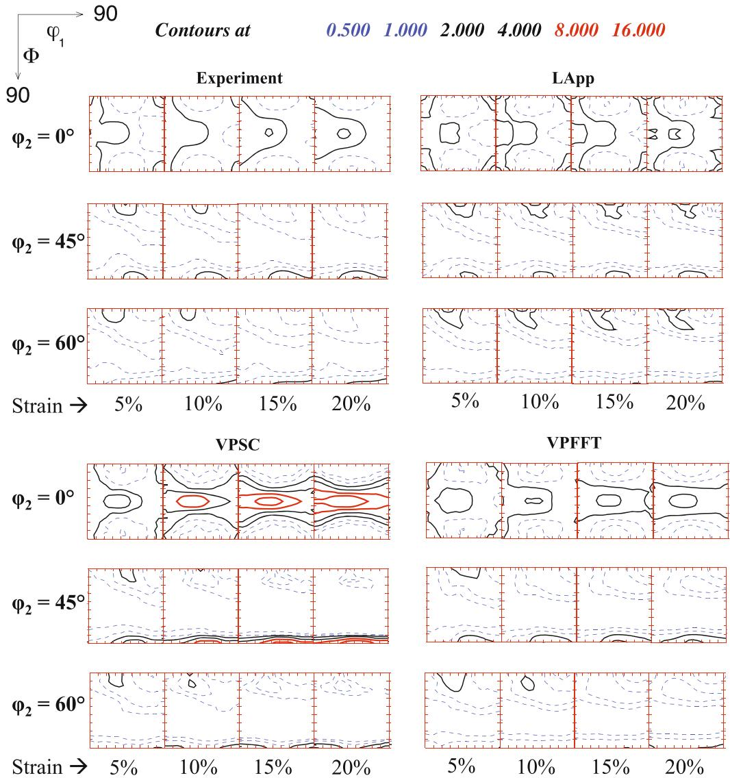
Fig. 14—Comparison of OD sections for equibiaxial stretch. The strain levels are 5, 10, 15, and 20 pct in RD (or TD, since strains in the two directions are the same).
