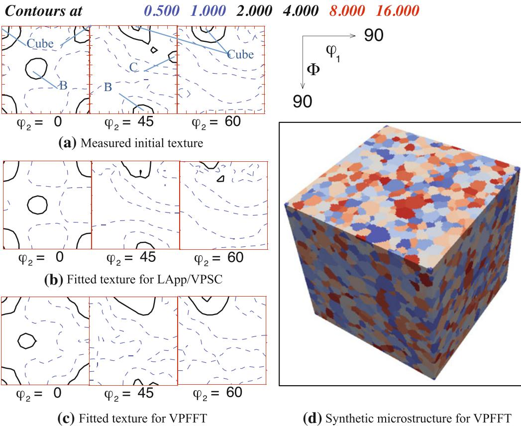
Fig. 1—Comparison of 0, 45, and 60 deg  $\varphi_2$  sections in (a) the experimental OD and fitted ODs for the (b) LApp, VPSC, and (c) VPFFT models. Locations of ideal texture components (Cube, Brass, and Copper) are noted. The unit for contour levels is multiples of random intensity. (d) The  $128 \times 128 \times 128$  synthetic microstructure for the VPFFT model with 5403 grains is shown. Colors denote different grains.
