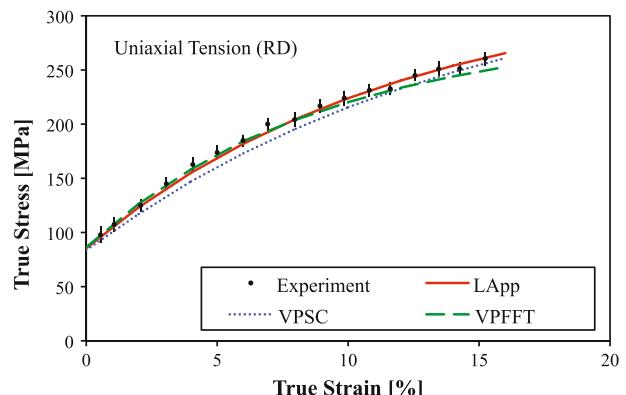
Fig. 4—Comparison of measured and simulated stress-strain curves for RD uniaxial tension.
