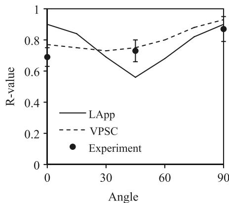
Fig. 20—Calculated  $R$  values vs the angle between the rolling direction and the stressing direction, with experimental values and error bars for comparison.
