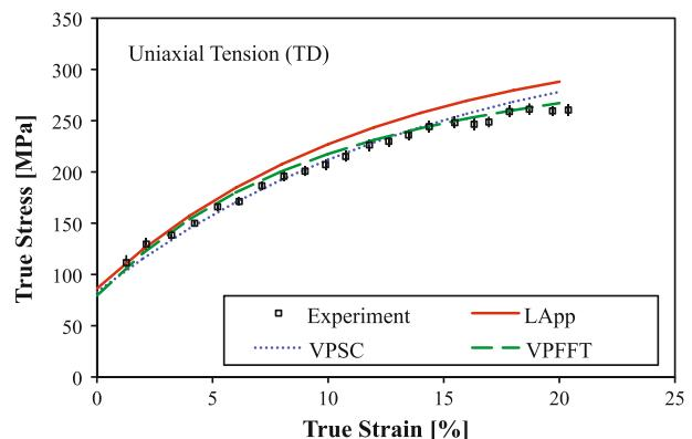
Fig. 5—Comparison of measured and simulated stress-strain curves for TD uniaxial tension.
