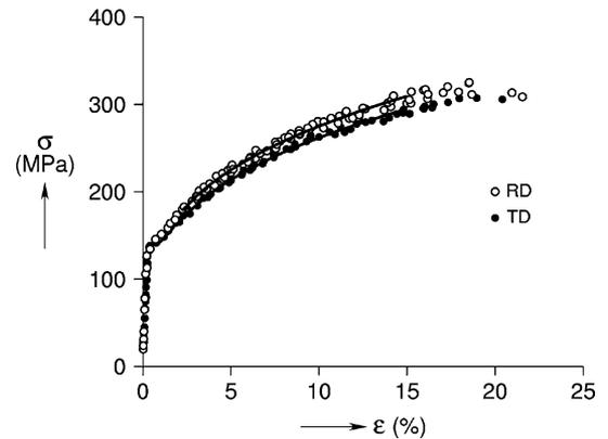
Fig. 5—*In-situ* uniaxial results (circles) with power-law fit curves.
