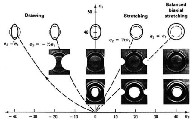
Fig. 1—Strain space description with images of the Raghavan-shaped specimen and matching washers.<sup>[6]</sup>
