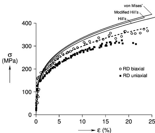
Fig. 10—Comparison of *in-situ* biaxial data in the rolling direction (open circles and dashed curve) and model predictions using the equivalent stress-strain construction and *in-situ* uniaxial power-law fit in the rolling direction.
