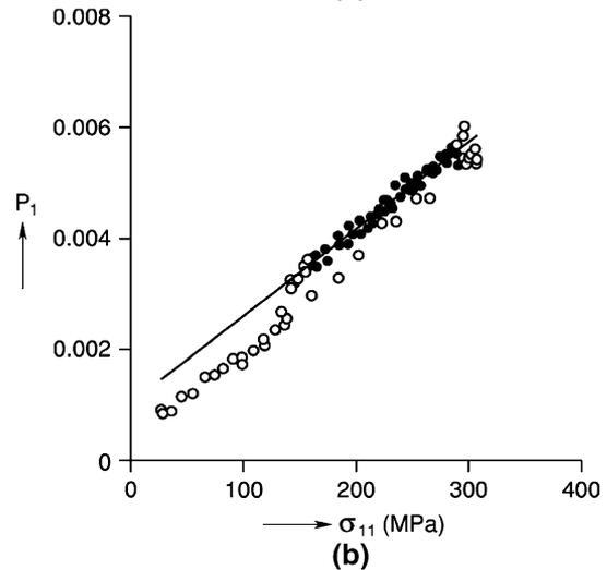
Fig. 7—Comparison of the slope ( $P_1$ ) of XRD measured lattice strain *vs*  $\sin^2\psi$  data and load cell measured stress for the *in-situ* uniaxial experiment in (a) the RD and (b) the TD. The slope of the linear fits shown here are the calibrated XECs,  $(1 + \nu)/E$ , for each orientation. Only the solid points are used in the linear regression.
