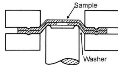
Fig. 2—Through section of Maciniak tooling with the Raghavan specimen and washer.
