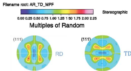
**Figure 4.** Recalculated  $\{111\}$  pole figures of as-received materials.
