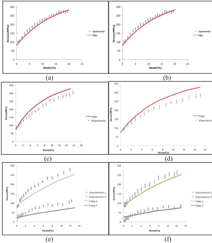
**Figure 2.** Comparison of stress-strain curves measured in the experiments and predicted by Taylor FC model using the LApp code for different strain modes. (a) RD-oriented and (b) TD-oriented uniaxial tension; (c) along the RD and (d) TD direction for equibiaxial stretch; (e) RD-oriented and (f) TD-oriented plane strain.
