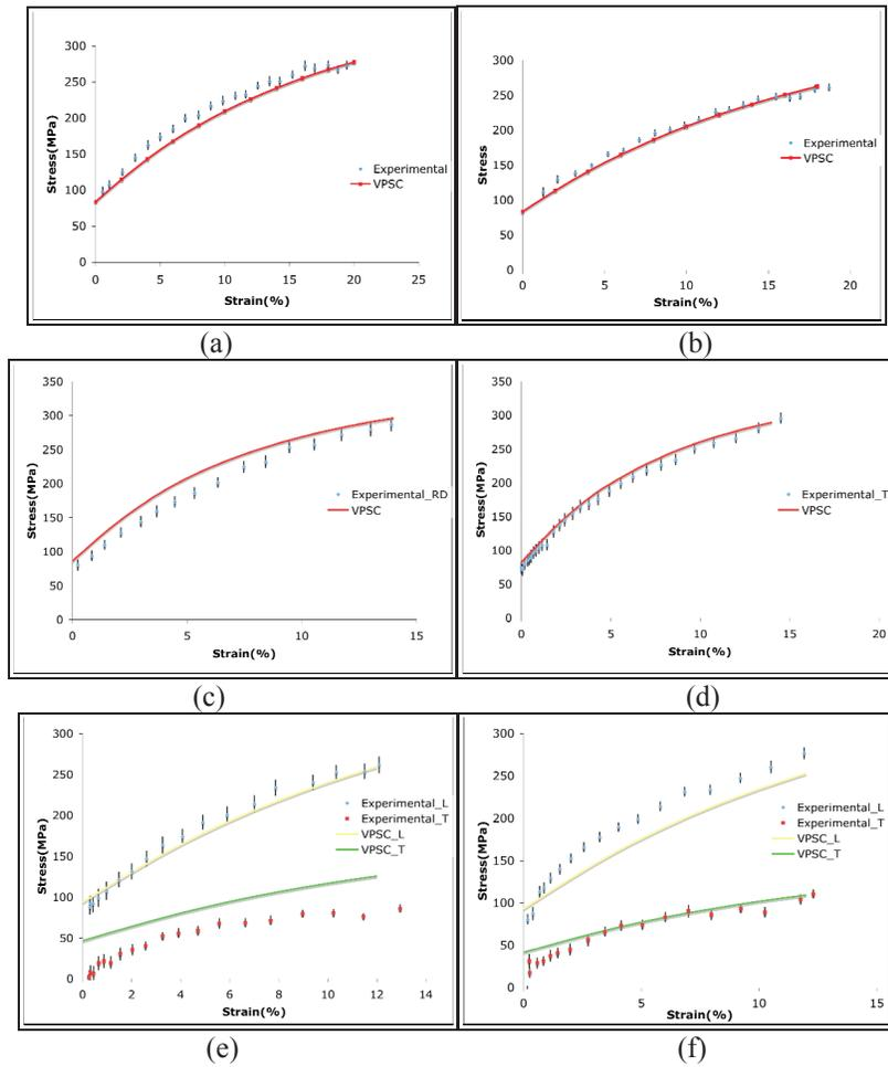
**Figure 3.** Comparison of stress-strain curves measured in the experiments and predicted by VPSC for different strain modes. (a) RD-oriented uniaxial tension; (b) TD-oriented uniaxial tension; (c) along the RD and (d) TD direction for equibiaxial stretch; (e) TD-oriented plane strain.
