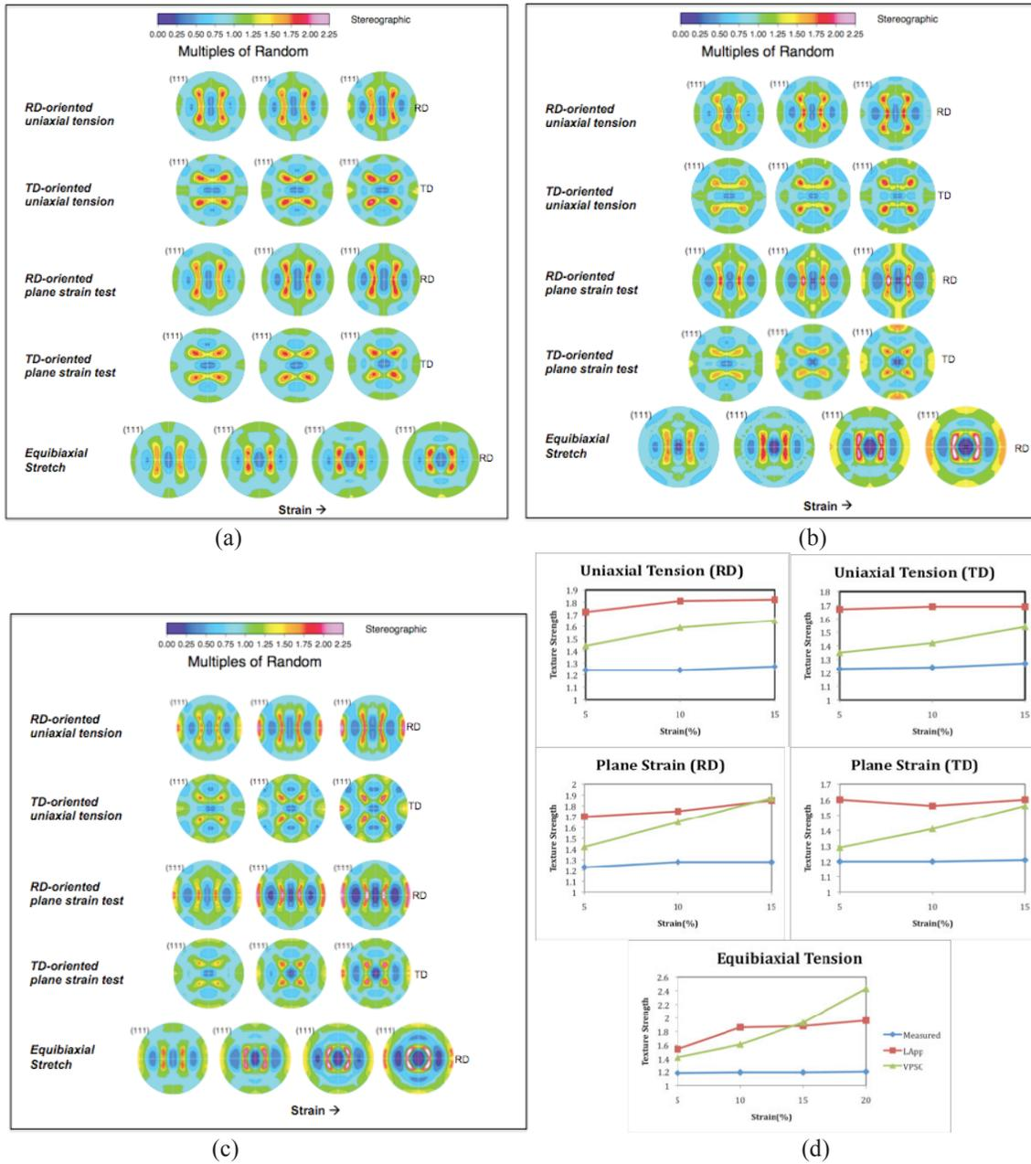
**Figure 5.** Evolution of  $\{111\}$  pole figures with strain level from (a) experiments and simulation by (b) *LApp* (c) and *VPSC*; in each figure, the strain levels 5%, 10% and 15% going from left to right, except for equibiaxial tension which also has 20%; (d) texture strength as a function of strain.
