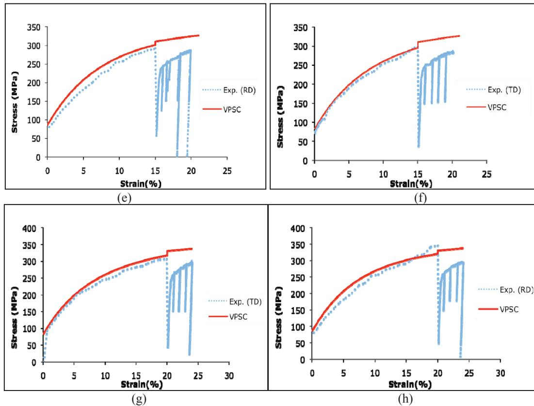
**Figure 6.** Comparison of stress-strain curves measured from experiments and simulated by VPSC for RD-oriented tension after (a) 5% (c) 10% (e) 15% (g) 20% biaxial prestrain; TD-oriented uniaxial tension after (b) 5% (d) 10% (f) 15% (h) 20% biaxial prestrain.
