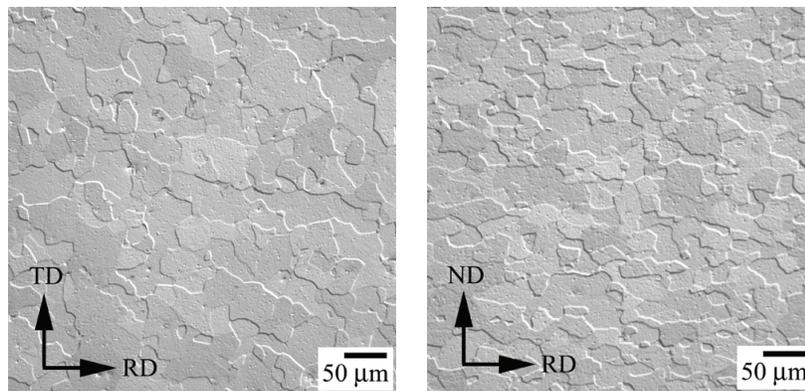
**Figure 1.** Optical micrographs of as-received AA5754 sheet material showing a nearly equiaxed microstructure in both RD-TD and RD-ND cross-sections [8].
