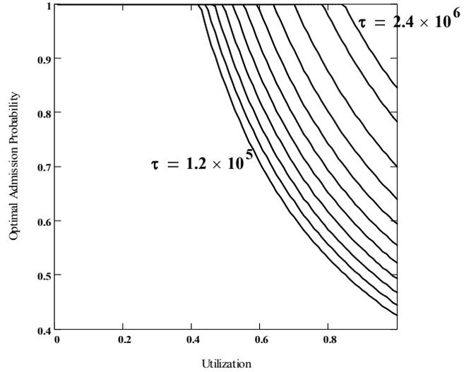
Figure 7. Optimal admission probability vs. utilization for varying decay rates.
