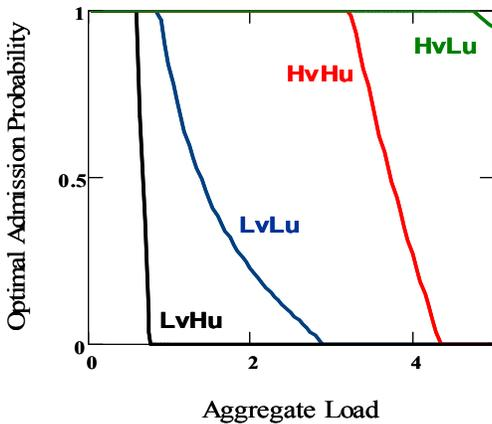
Figure 15. Optimal admission probability vs. aggregate load for simulated job classes described in Table 2.
