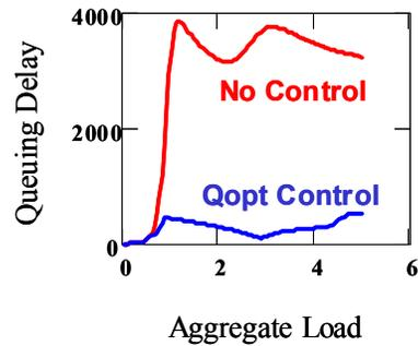
Figure 18. Average queuing delay vs. aggregate load when admitting all jobs (red) and when applying optimal admission probabilities (blue).
