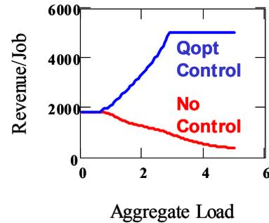
Figure 17. Average revenue per job vs. aggregate load when admitting all jobs (red) and when applying optimal admission probabilities (blue).
