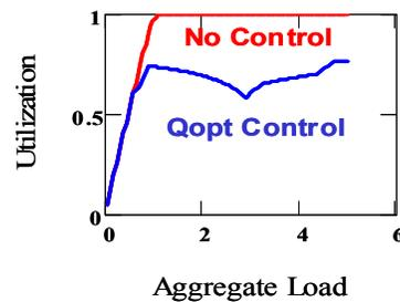
Figure 19. Average utilization vs. aggregate load when admitting all jobs (red) and when applying optimal admission probabilities (blue).
