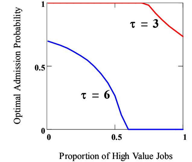
Figure 10. Optimal admission probability for varying proportion of high-value jobs given utilization of 80% ( $\tau$  is in units of  $10^5$ ).
