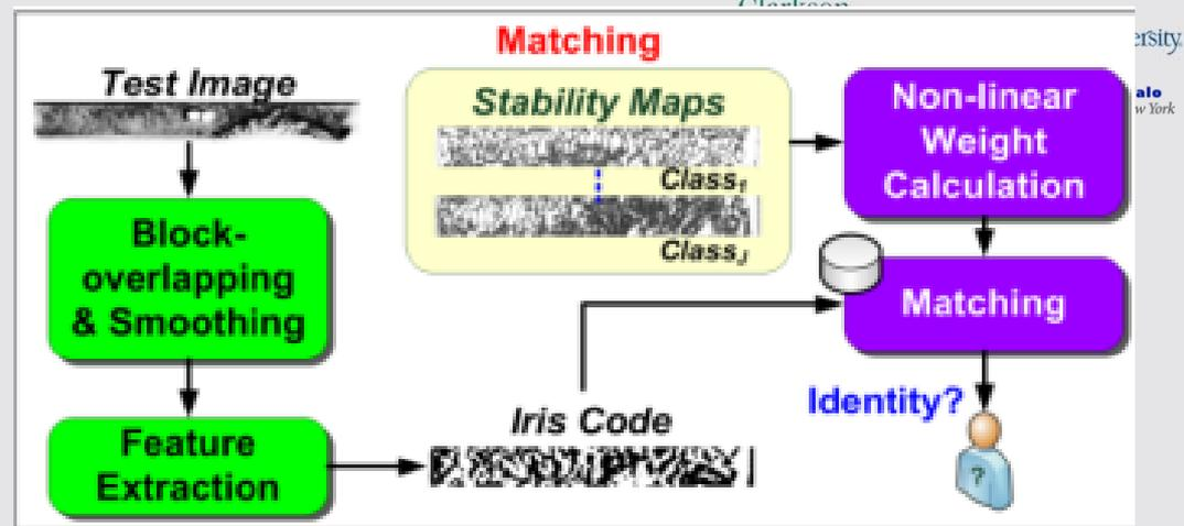
Figure. Block diagram of the developed iris recognition scheme. (a) Stability maps learning phase, (b) Matching phase.
