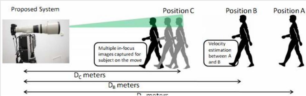
*Figure. Subject approaches the system, crosses variable checkpoints A and B, estimates his/her speed. Focus position is then set to a position C to obtain an iris of required resolution. A number of in-focus images are then acquired by changing the focus continuously based on subject distances estimated.*
