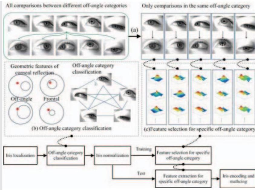
Figure. The flowchart of off-angle iris recognition using Corneal reflections and multiclass SVM
