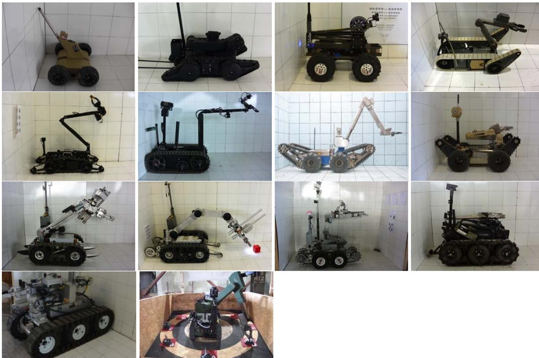
**A wide variety of ground robots** used during C-IED training exercises show how different sizes and configurations of robots could be applicable. They included some new robots provided by manufacturers, showing how standard test methods can also provide good teaching aids to learn new robot interfaces and capabilities.
