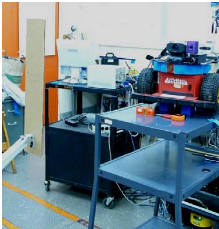
Figure 4 – Small robot vehicle on a cart in front of the large robot vehicle. Left shows the rear of the flat target being supported from the test stand. The large black camera was not used. Note the blue tape covering all except the front facing sonar sensor.
