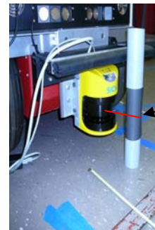
Figure 5 – Optical 2D scanning LADAR sensor mounted on the large vehicle with the 70 mm dia. x 400 mm long test piece set in front and covered with a piece of black standard reflectance paper.
