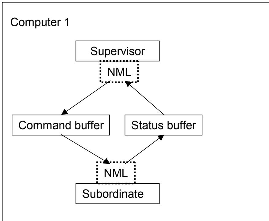
There are two NML buffers, each with a single reader and a single write. The supervisor writes the command buffer, and the subordinate reads it. The supervisor reads the status buffer, and the subordinate writes it. NML ensures mutual exclusion for data consistency.
