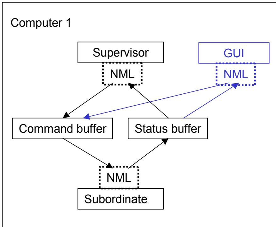
A graphic user interface (GUI) has been added. Now, the command buffer has two writers, and the status buffer has two readers. NML ensures mutual exclusion, as before.
