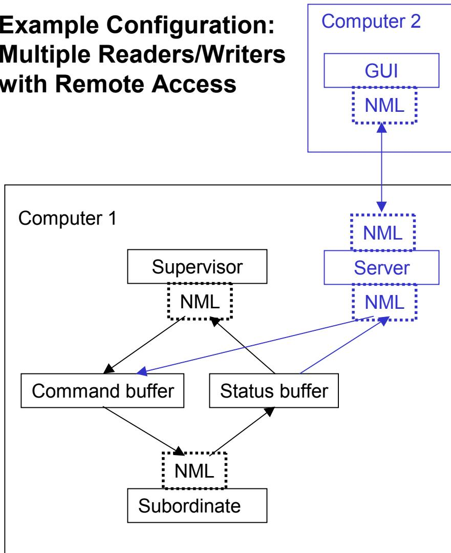
GUI has moved to Computer 2. System now requires an NML server on Computer 1, which mediates read and write requests from the GUI. Communication between the GUI and the server is accomplished using TCP/IP sockets. The server accesses the target command and status buffers locally, as the GUI did before.
