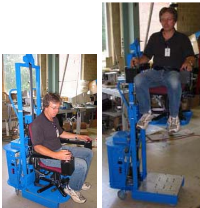
RoboChair 1 demonstrated patient mobility with skid-steer control and lift of approximately 1 m high while seated in the chair attached to the lift structure. The unit included front skid-steered drive wheels with drive motors beneath the lower plate. The rear housed batteries and control electronics.
