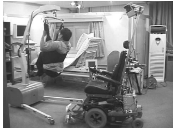
(left) Autonomous moving to the predefined position, (right) Docking operation
