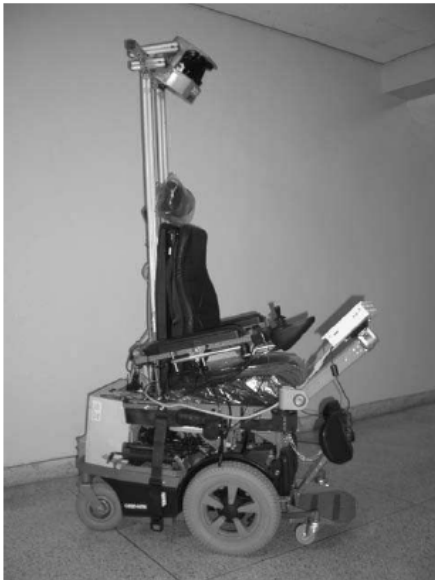
(left) Robotic Wheelchair Platform, (right) Hierarchical Control Architecture of the System
