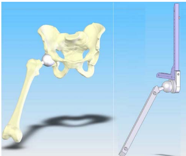
Figure 1. The image on the left is a depiction of a patient pelvis along with a femur bone and an artificial ball joint. Comparing this to the NIST phantom and femur bar on the right side of the figure, it is easy to recognize the motivation for the construction of the measurement artifact.
