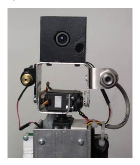
Figure 6: The main camera with thermosensor
