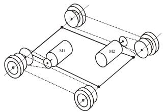
Figure 2: Simplified scheme of the locomotor
