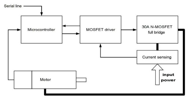
Figure 5: Block diagram of control and power switching board
