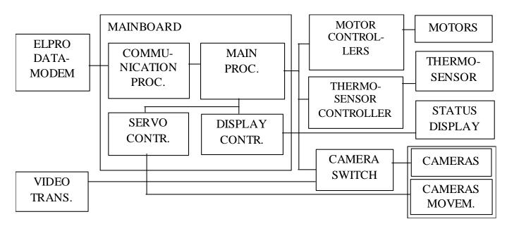
Figure 4: Electronics subsystem scheme
