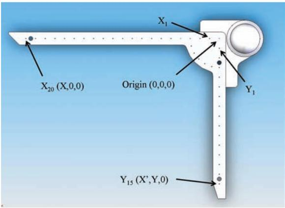
The L shape XY coordinate frame with the target holes
