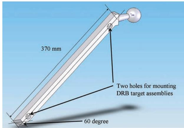
nominal distance can be calculated assuming a nominal increment of 15 mm, between neighboring holes, the actual distance is determined through careful calibration to be described in a future paper.
