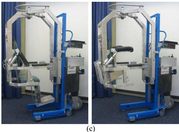
Figure 4 – Graphics of the HLPR Chair (a) approaching and placing a person on a toilet and showing length dimensions, and (b) placing a person on a comfortable chair. (c) Photographs of the HLPR Chair in the same positions as in the center and right graphic (a).
