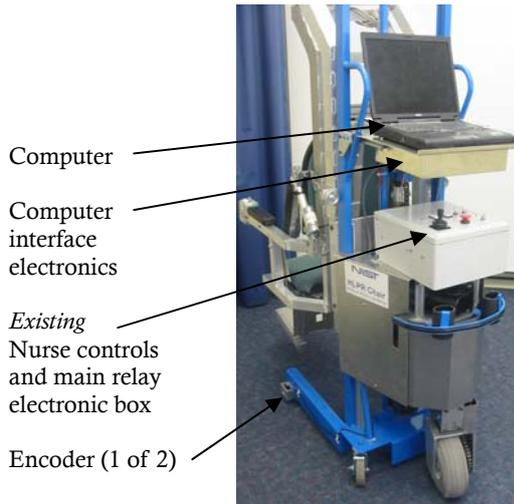
Figure 6 – Photograph of the HLPR Chair with recently added front wheel encoders, development computer and interface electronics, and advanced 3D imaging camera and color camera (cameras are shown in Figure 1).
