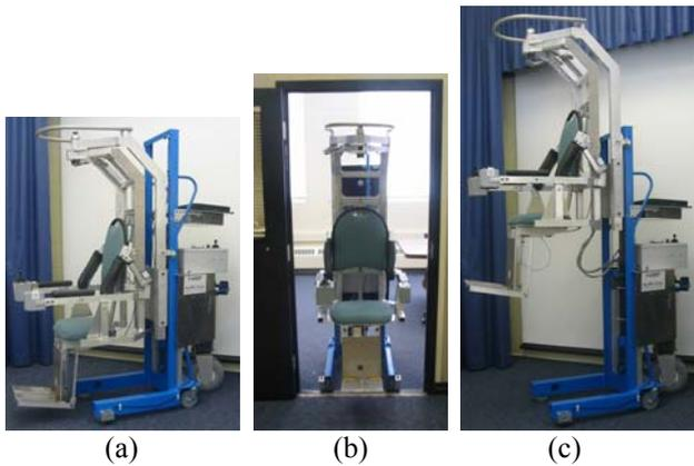
Figure 2 – Photographs of the HLPR Chair in the mobility configuration showing the (a) side view and (b) front view relative to a typical doorway and (c) the lift configuration. The maximum patient lift height is 0.9 m (36 in) above the mobility height configuration.
