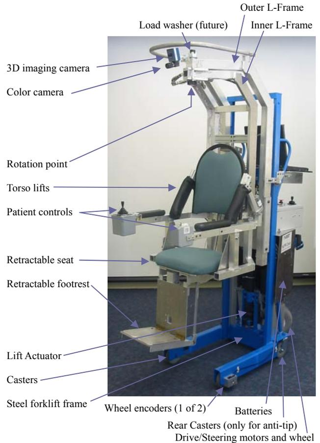
Figure 1 –Photograph of the HLPR Chair prototype.
