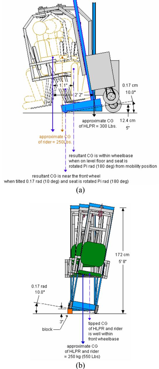
Figure 3 – CAD models of the HLPR Chair testing static stability in the (a) forward and (b) sideways directions approximating maximum tipping angles for each.
