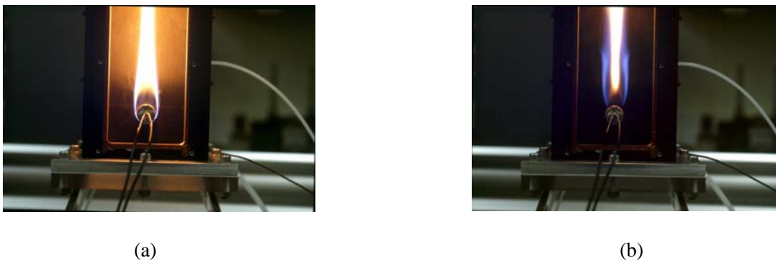
Figure 4. (a) An enveloped flame and (b) a wake flame.
