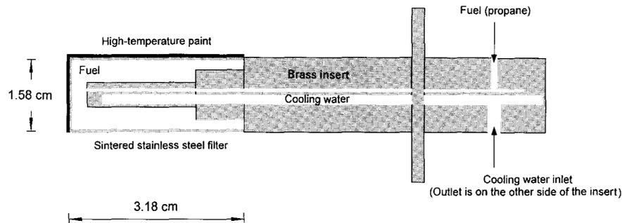
Fig. 2. A cut-away view of the burner insert.
