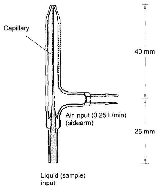
Fig. 3. A schematic representation of the nebulizer.
