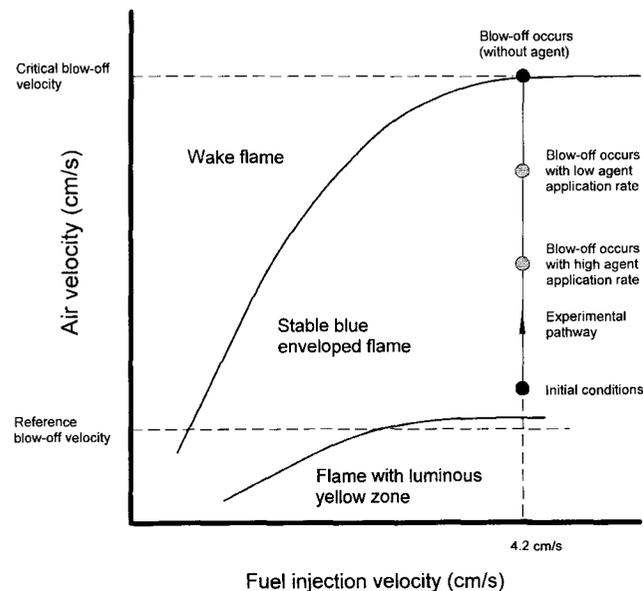
Fig. 8. A schematic representation illustrating the experimental procedure.
