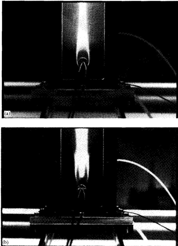
Fig. 4. Photographs of an enveloped flame (a) and a wake flame (b).
