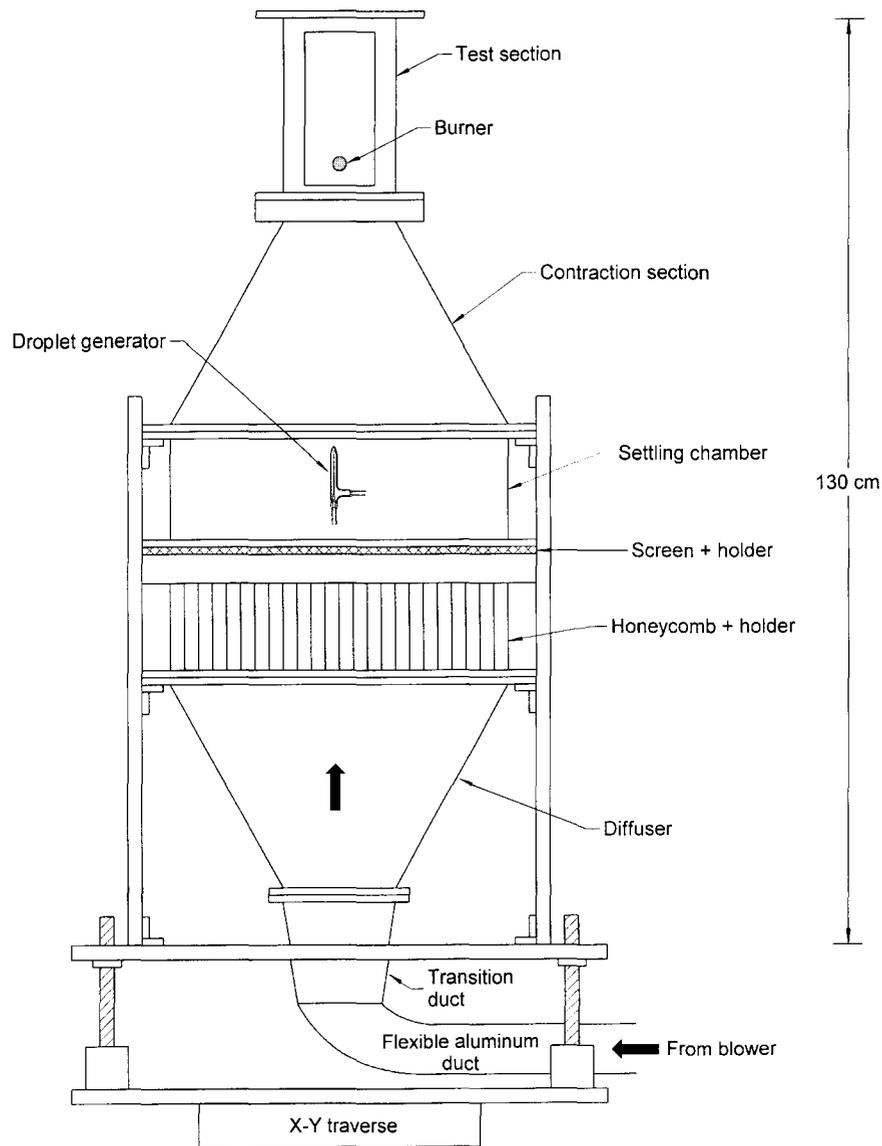
Fig. 1. A schematic representation of the wind tunnel.
