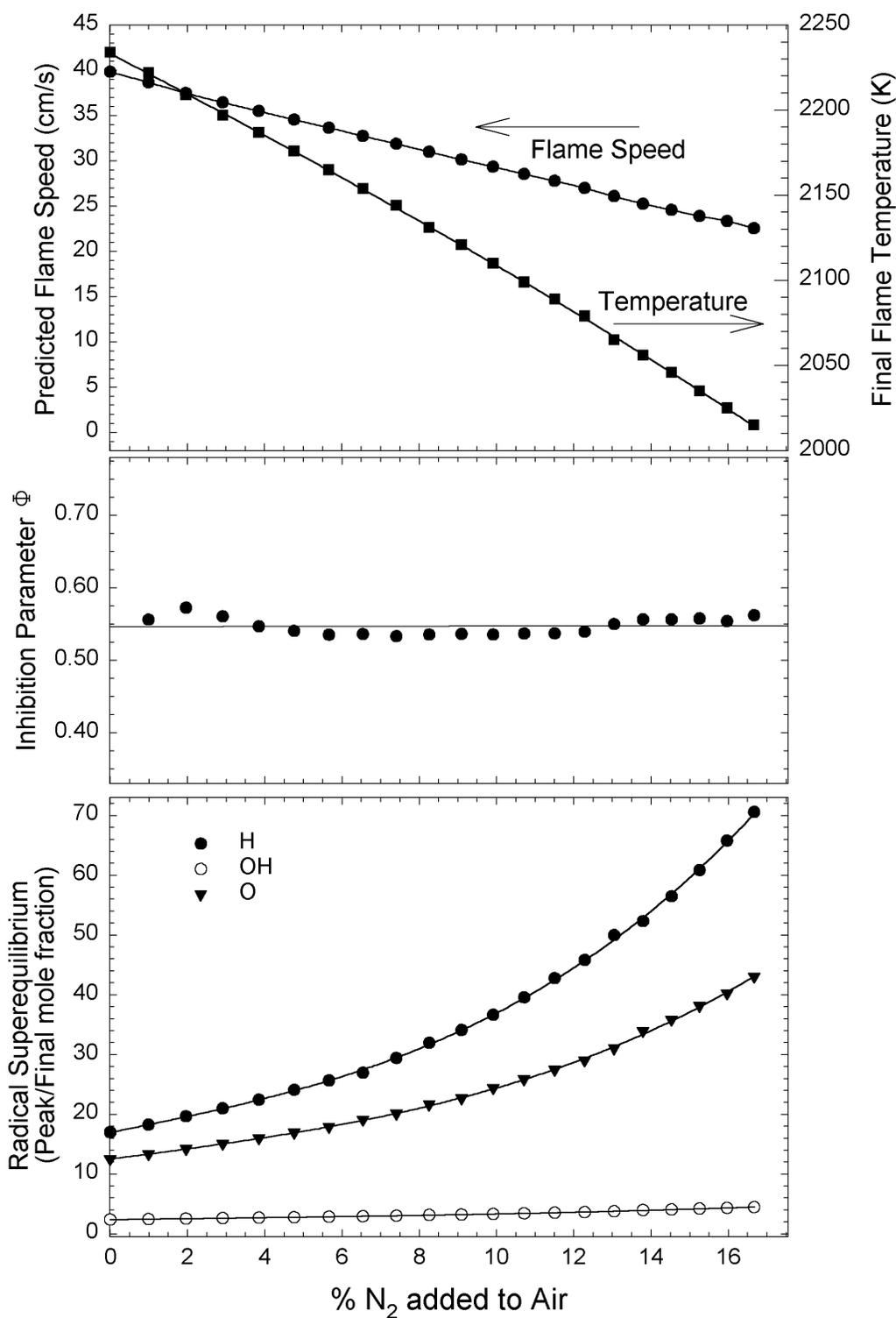
Figure 1: Flame speed, final flame temperature, inhibition parameter (defined in Ref. [3]), and superequilibrium concentrations of flame radicals computed for atmospheric pressure stoichiometric methane/air mixtures inhibited by nitrogen.
