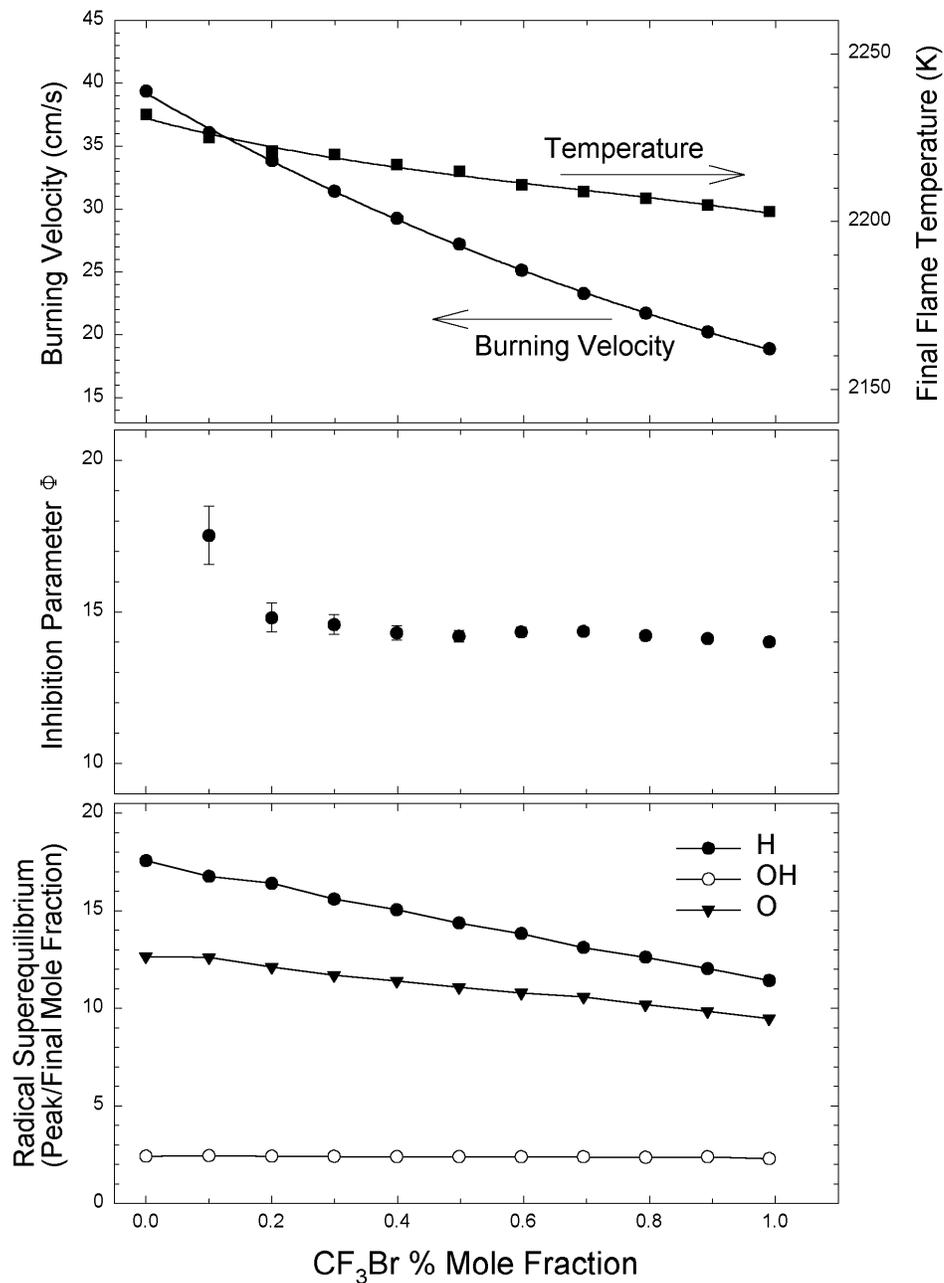
Figure 3: Flame speed, final flame temperature, inhibition parameter (defined in Ref. [3]), and superequilibrium concentrations of flame radicals computed for atmospheric pressure stoichiometric methane/air mixtures inhibited by CF<sub>3</sub>Br.
