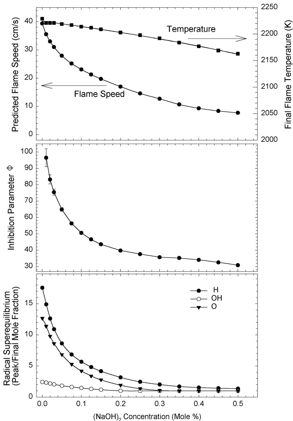
Figure 2: Flame speed, final flame temperature, inhibition parameter (defined in Ref. [3]), and superequilibrium concentrations of flame radicals computed for atmospheric pressure stoichiometric methane/air mixtures inhibited by sodium hydroxide. To simulate the evaporation process, NaOH was added to the reactants as a dimmer and required to undergo an endothermic decomposition process before inhibition chemistry could occur.
