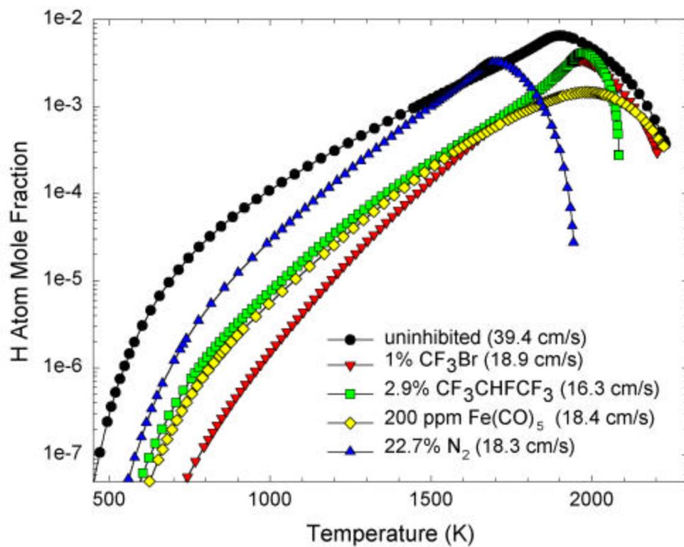
Figure 5: Mole fraction of atomic hydrogen as a function of local flame temperature for an uninhibited atmospheric pressure methane/air flame, and the same flame inhibited by various classes of suppression agents.
